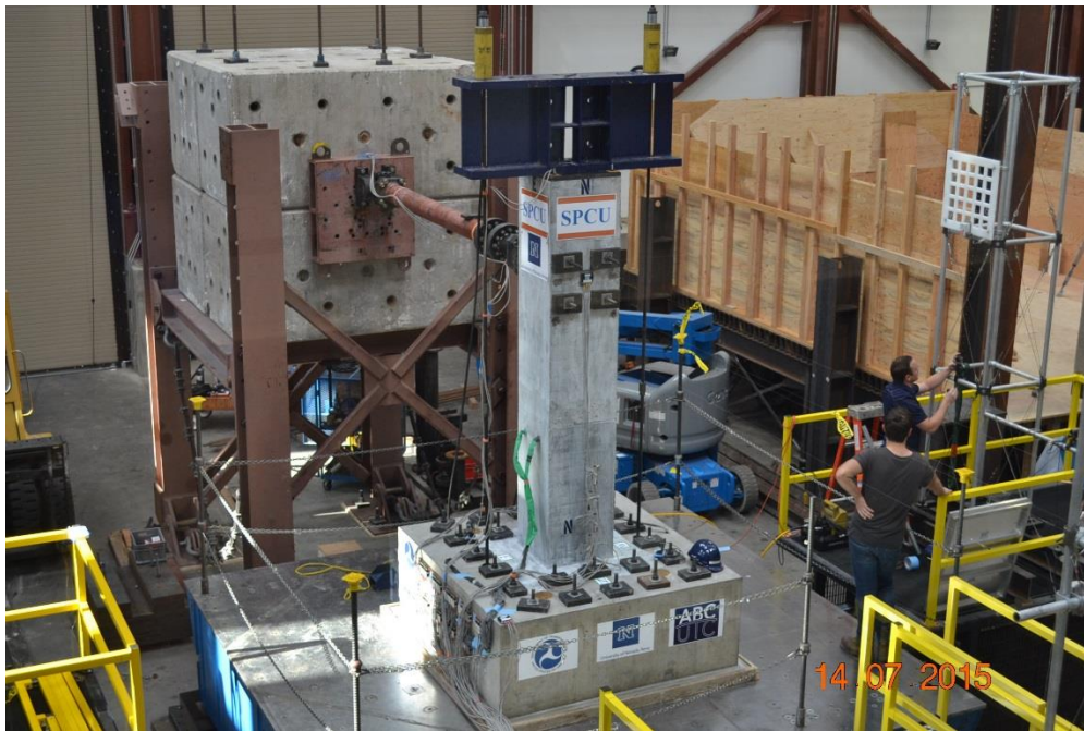
Column on a shake table at UNR
