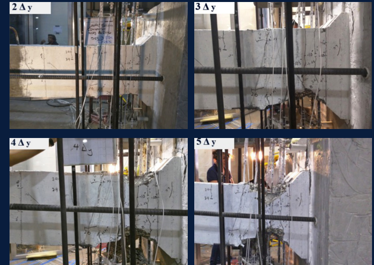
Connection damage at different displacement levels.
