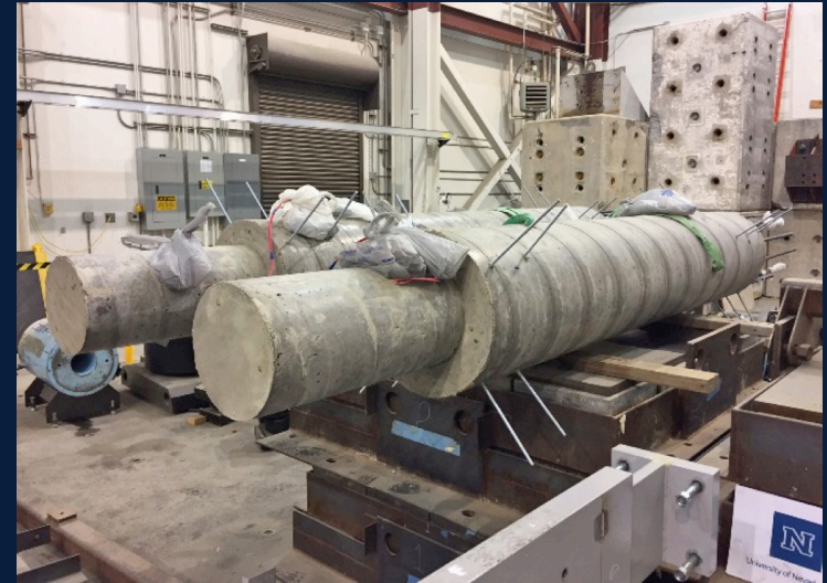
Precast columns for the two-column bent model of the bridge.
