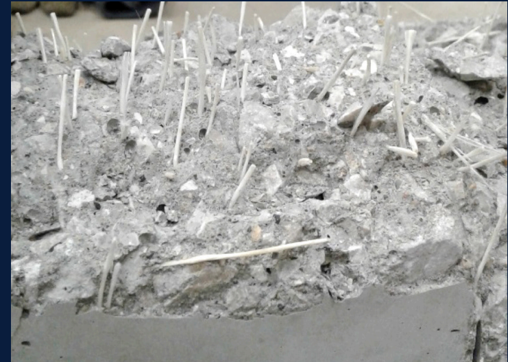
Fiber reinforced concrete after characterization for use in ABC link slabs.
