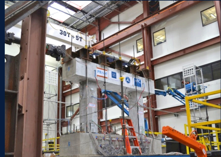
Two-column bent model shake table test setup.
