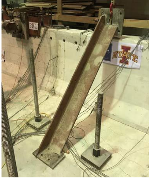
Figure 24 Beam used to brace the u-bar connected barrier during Test 4
