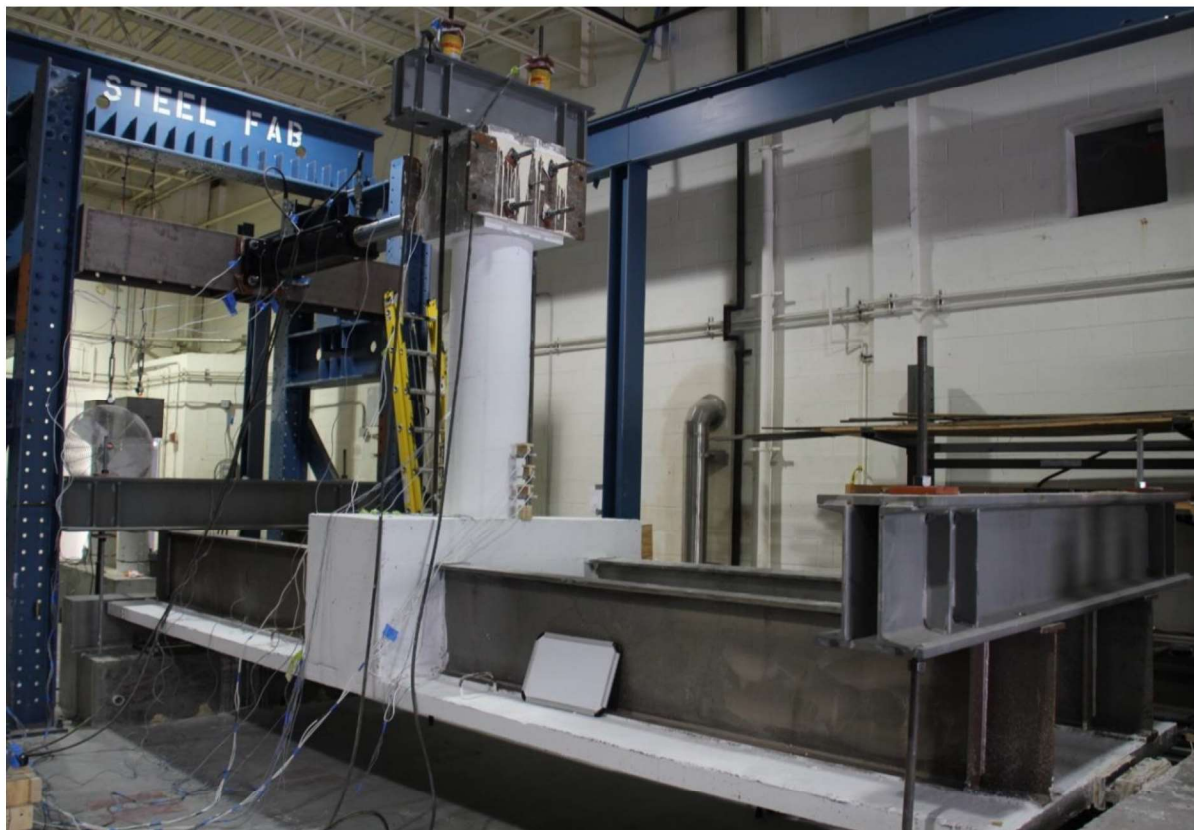
Figure 3-21 Component test set up before testing.
