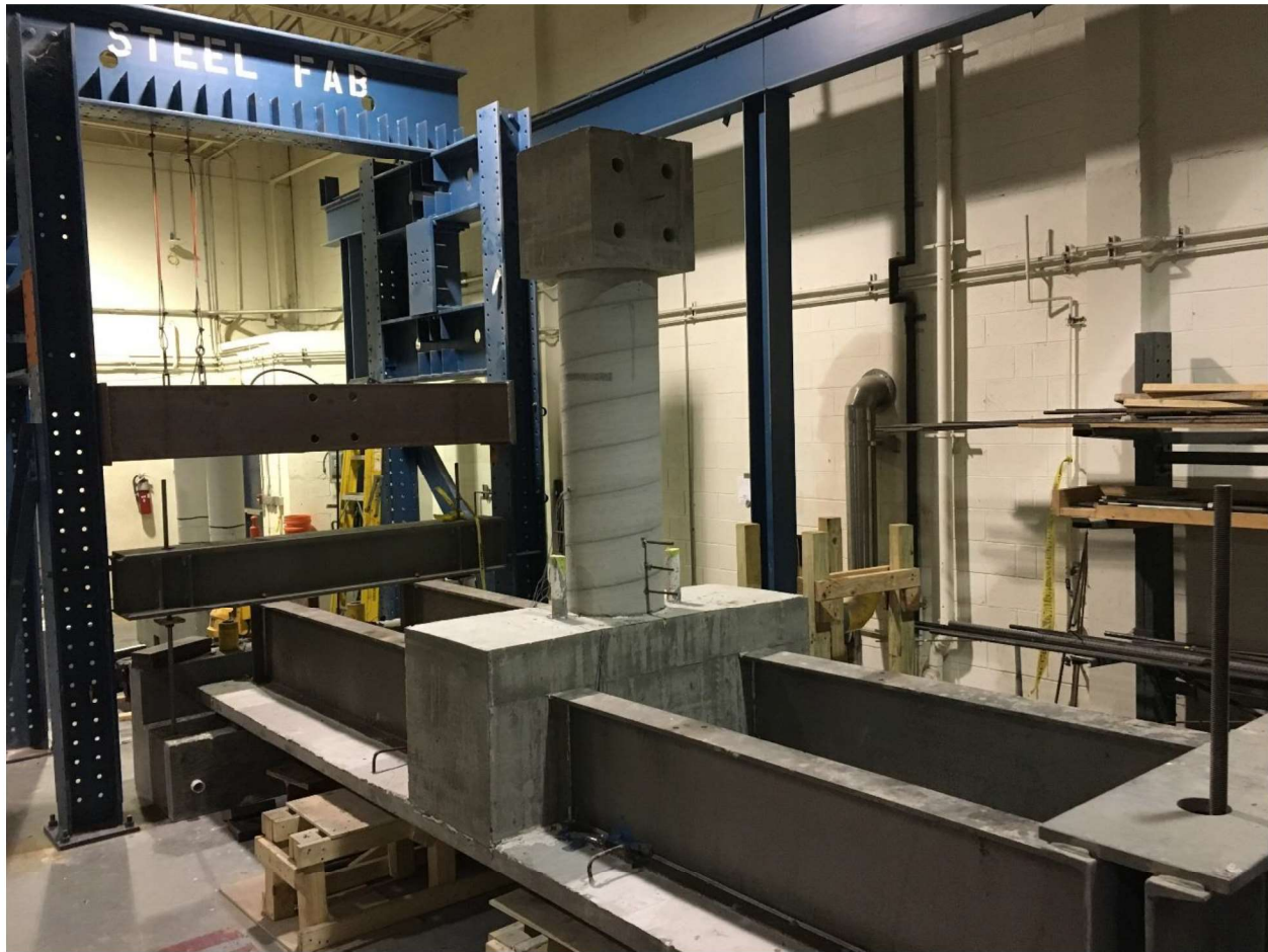
Figure 3-28 Test specimen after construction and removing formworks.
