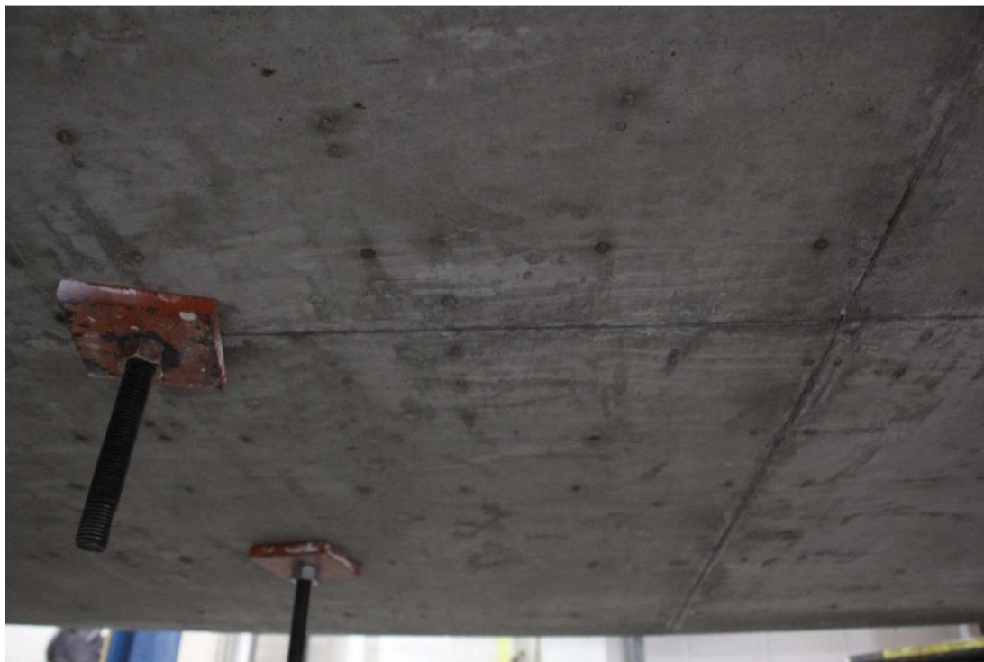
Figure 4-13 Bottom of the deck at the end of the test.
