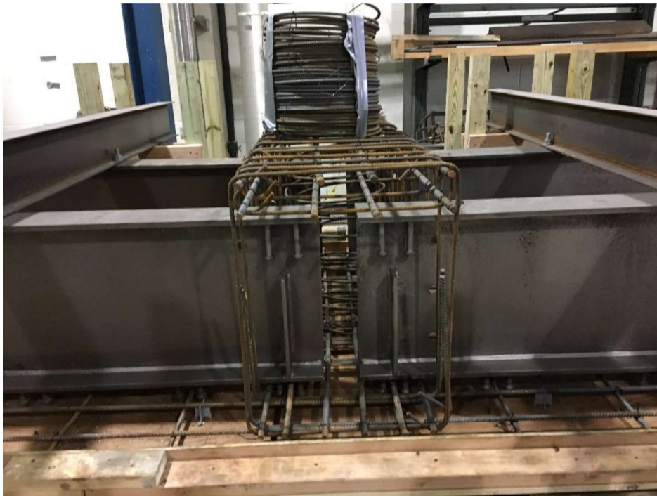
Figure 3-23 Specimen before casting step 1.
