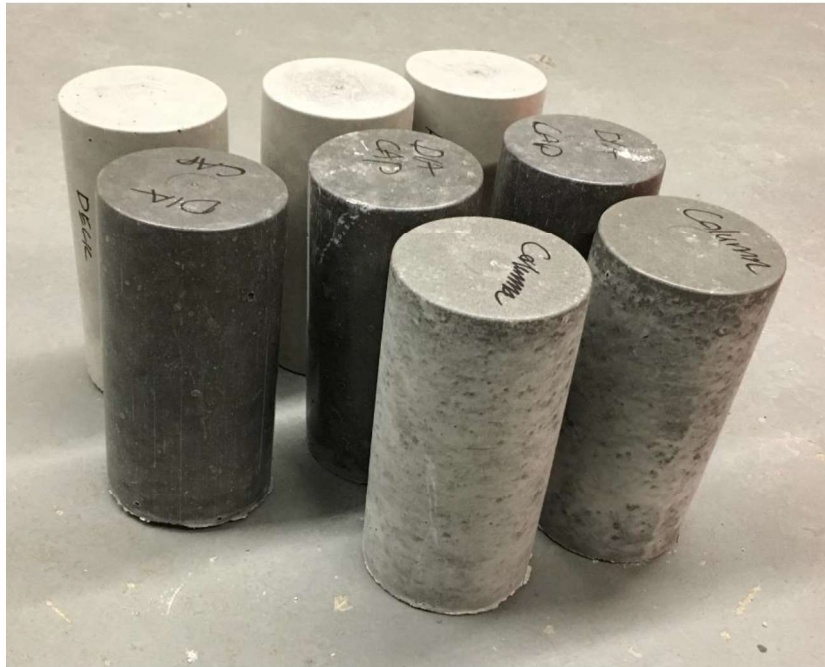
Figure 4-1 Sample concrete cylinders.
