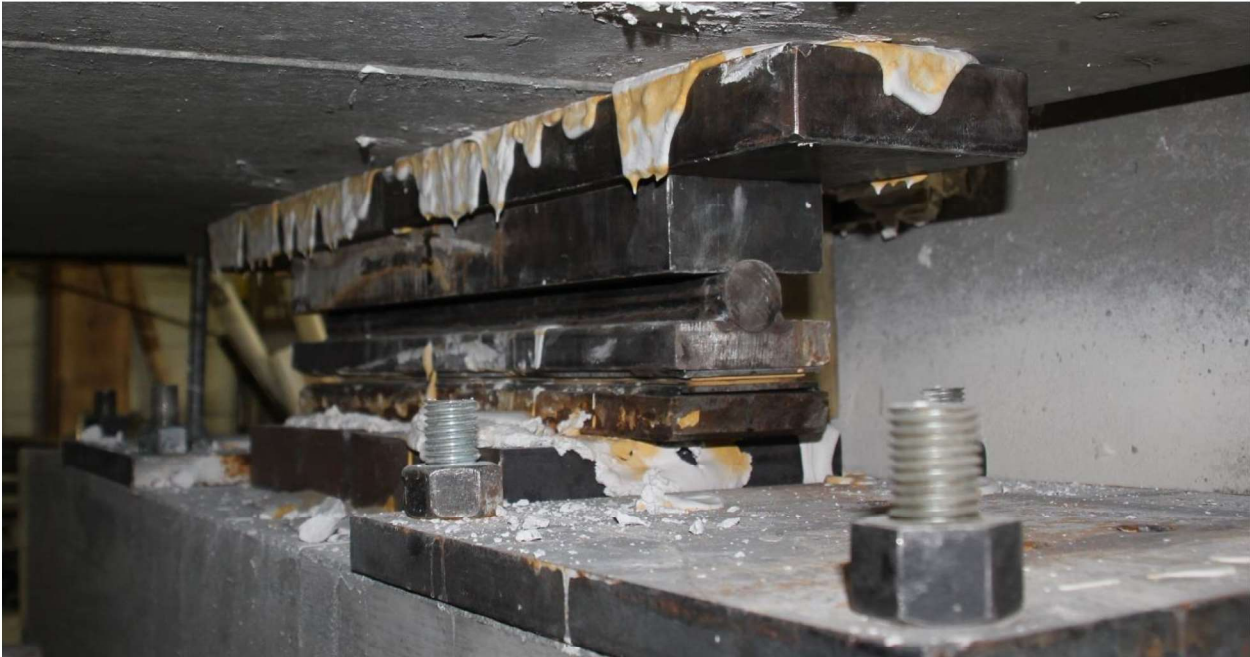
Figure 3-18 Roller support under the specimen.
