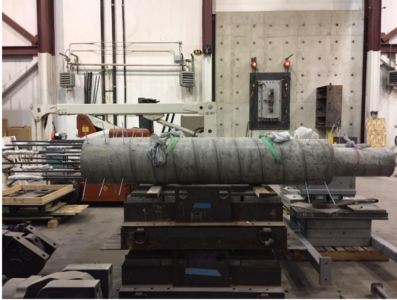
Fig. 45- Completed precast columns for the bent
