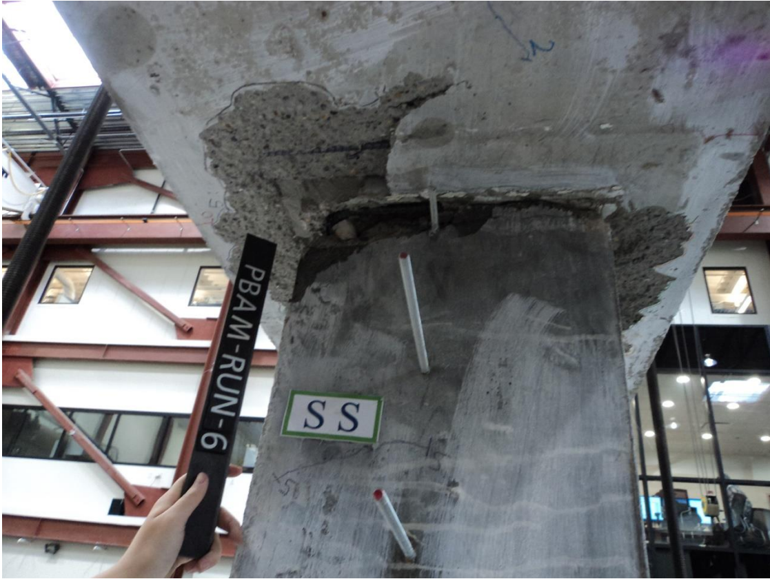
Figure 41. Damage state of UHPC plastic hinge and pocket connection under 150% design motion
