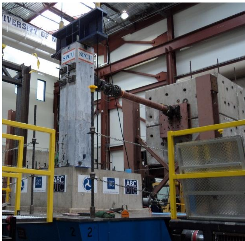
Figure 24. Shake table test set up
