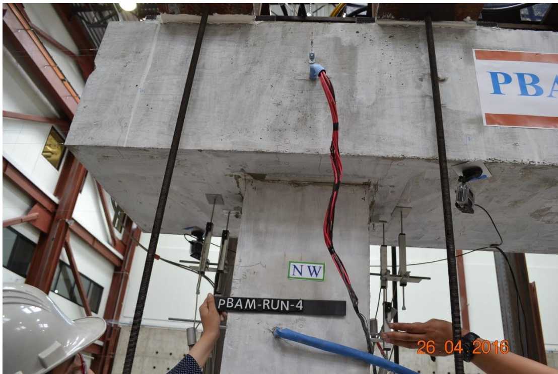
Figure 37. Damage state of ECC plastic hinge and pocket connection under design motion
