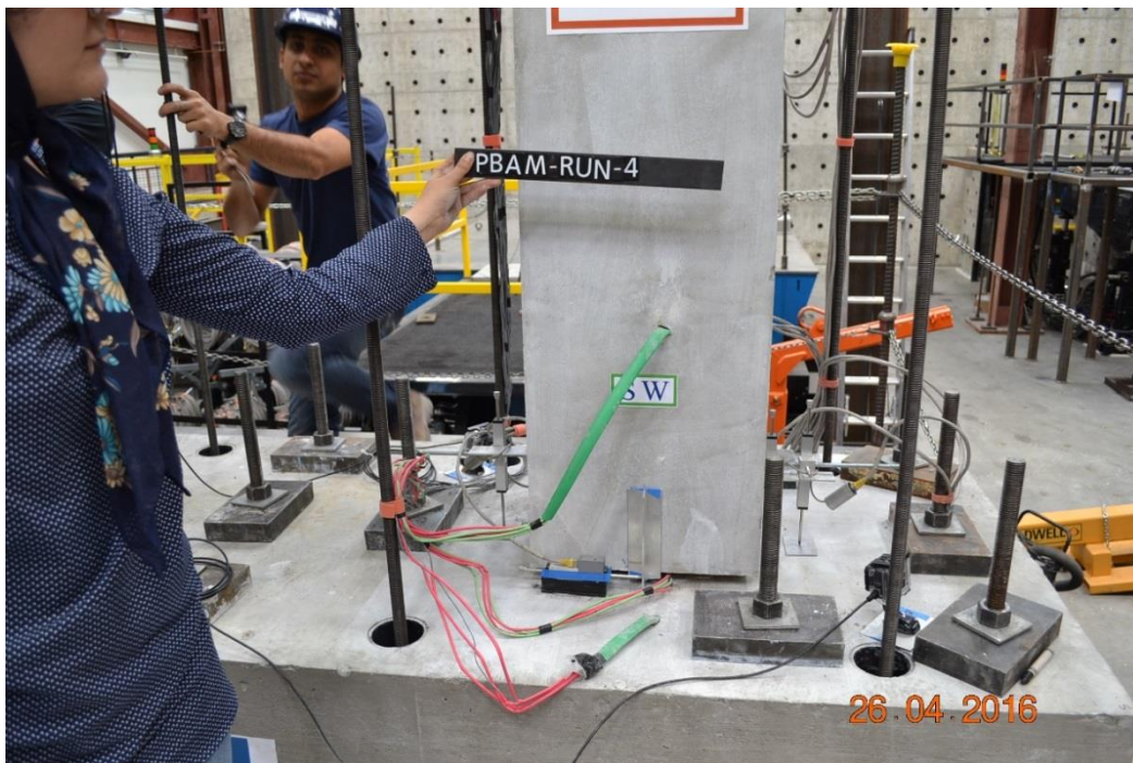
Figure 39. Damage state of two-way hinge under design motion
