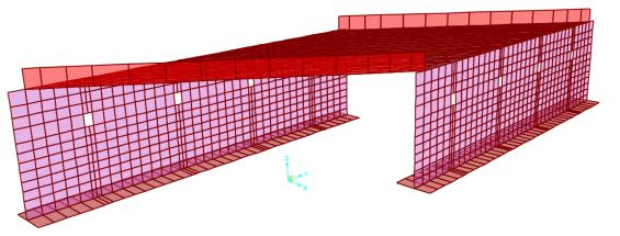
Concrete Rigid Frame Modeling – Shell Element
