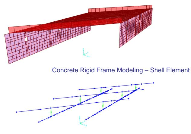
Transport System Modeling – Beam Element
