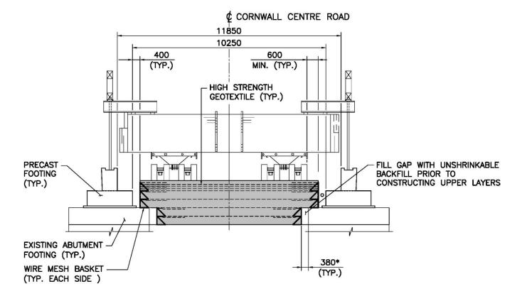
\* 150mm AT MEDIAN RETAINING WALL FOOTINGS GRANULAR B TYPE III TO BE COMPACTED TO 95% SPMDD GRANULAR A TO BE COMPACTED TO 100% SPMDD
