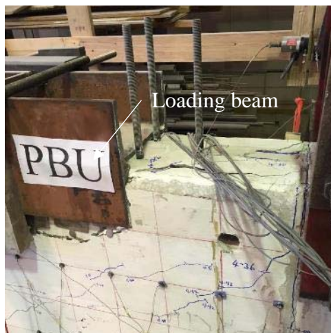
Figure 28 Cracking on barrier due to loading during Test 4
