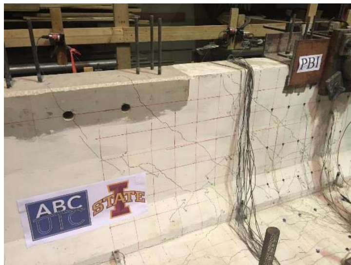
Figure 26 Diagonal cracks during Test 3
