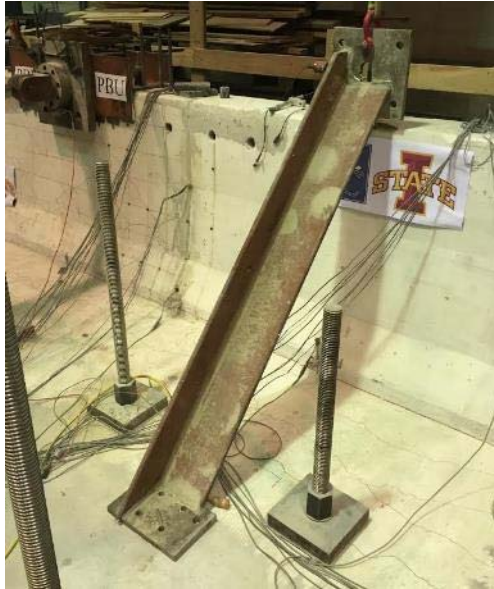
Figure 27 Beam used to brace the u-bar connected barrier during Test 4
