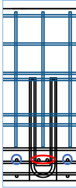
Figure 24 Schematic Drawing of Deck Reinforcement of U-bar
