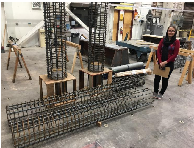
Fig. 42 – Column reinforcement cages
