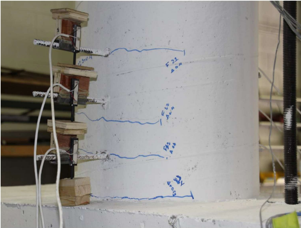
Figure 4-3 Forming of first cracks in the North side of the column
