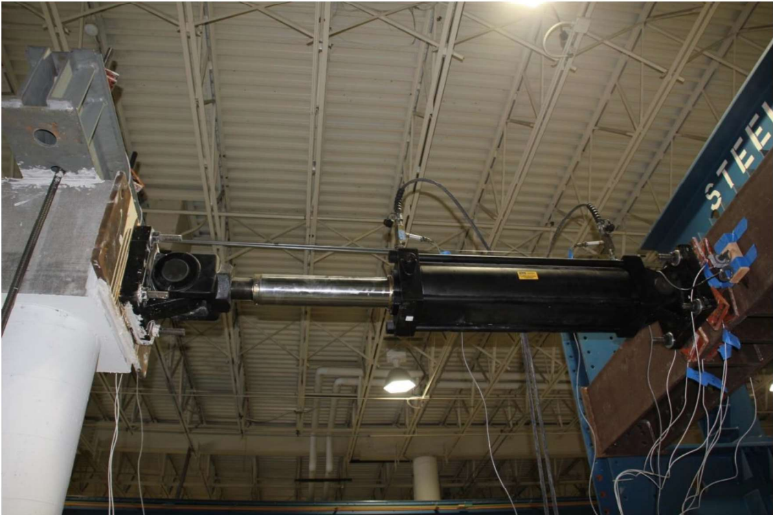
Figure 3-30 Hydraulic jack for applying lateral load.
