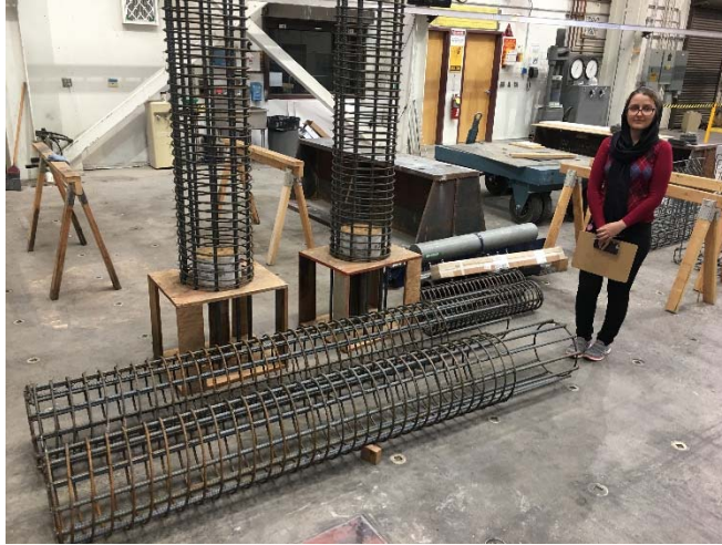
Fig. 43 – Column reinforcement cages
