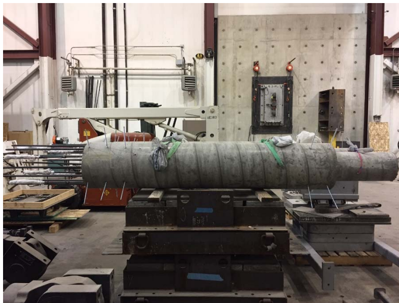
Fig. 46- Completed precast columns for the bent
