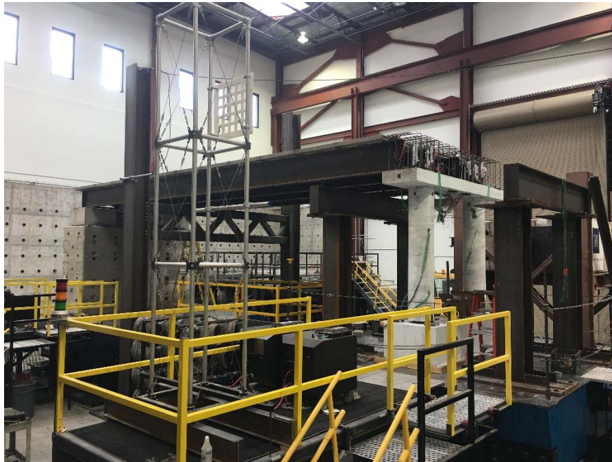
Fig. 61- The east span supported on east abutment and near the pier.
