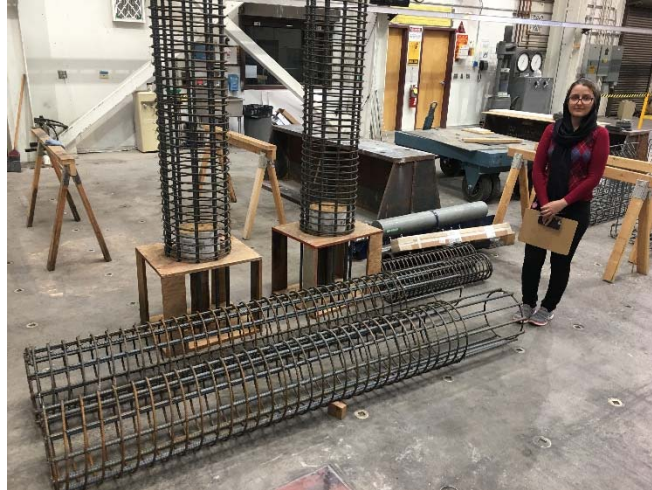
Fig. 43 – Column reinforcement cages
