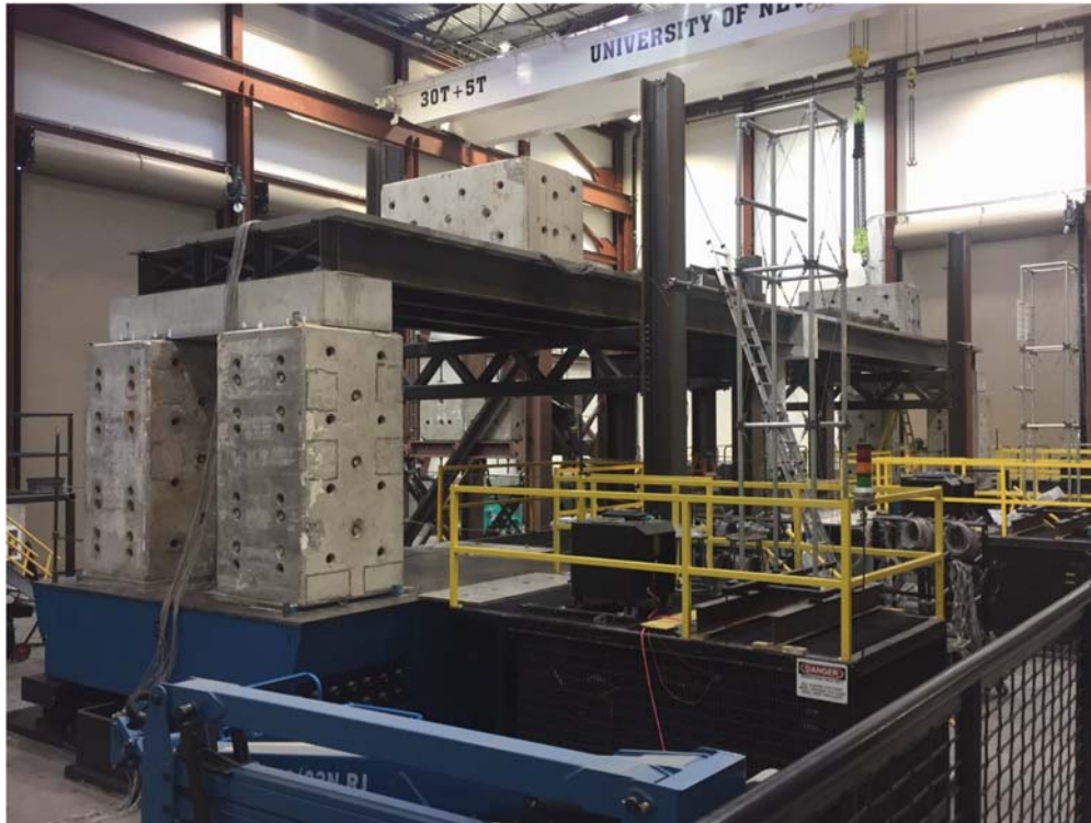
Fig. 62- Completed bridge model
