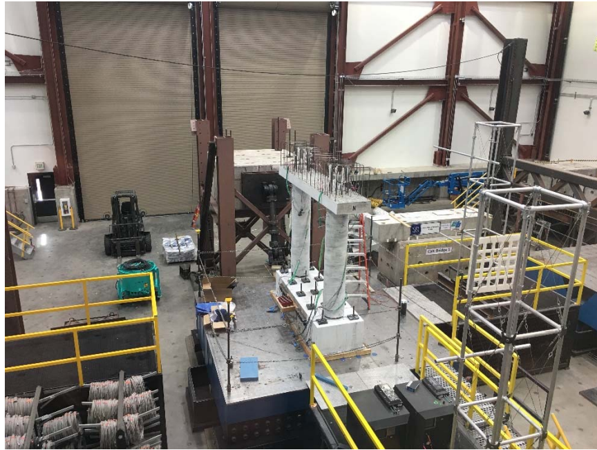
Fig. 60- Two-column bent secured to the shake table
