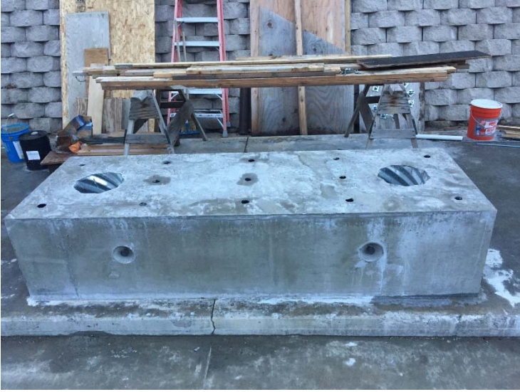
Fig. 45- Precast footing with sockets (pockets).
