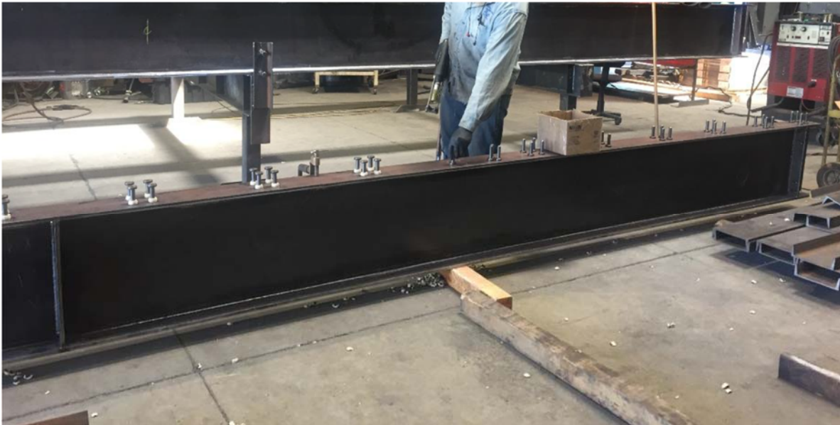
Fig. 53 –Attachment of studs
