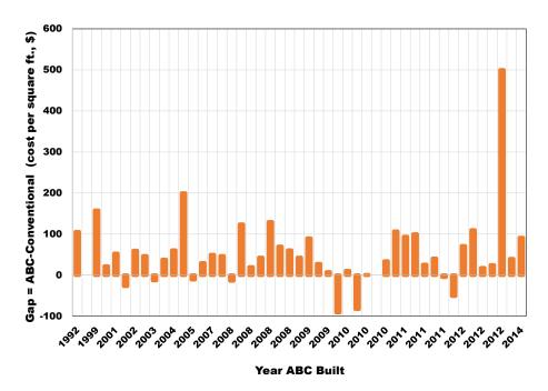
Figure 1. The comparison of ABC vs. the conventional construction cost estimates (Top) Comparison of construction cost of conventional and ABC bridges, (Bottom) The difference between ABC and conventional construction cost
