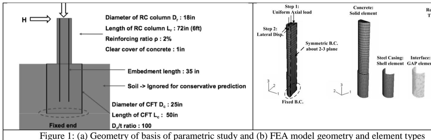
Figure 1: (a) Geometry of basis of parametric study and (b) FEA model geometry and element types
