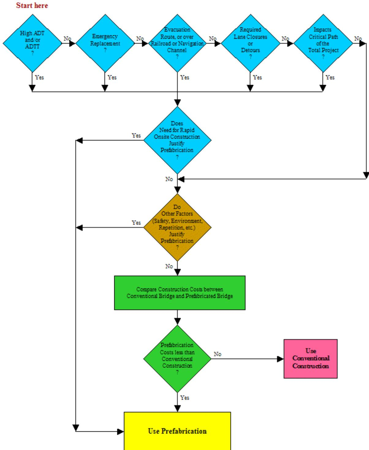
Figure 1: Decision-making flowchart to use prefabricated elements in bridge construction [1]
