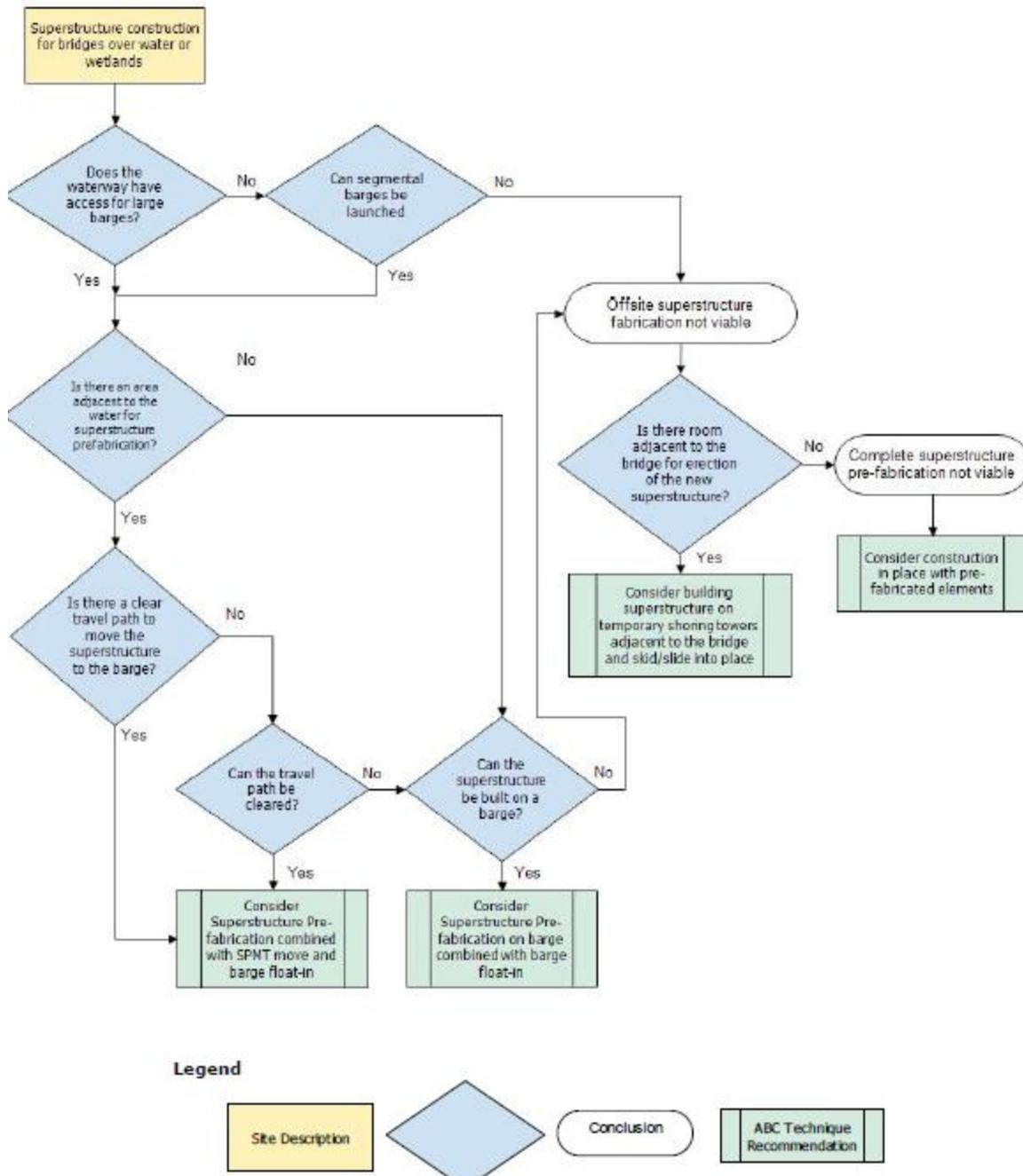
Figure 5: Decision flowchart for superstructure construction over the water [2]
