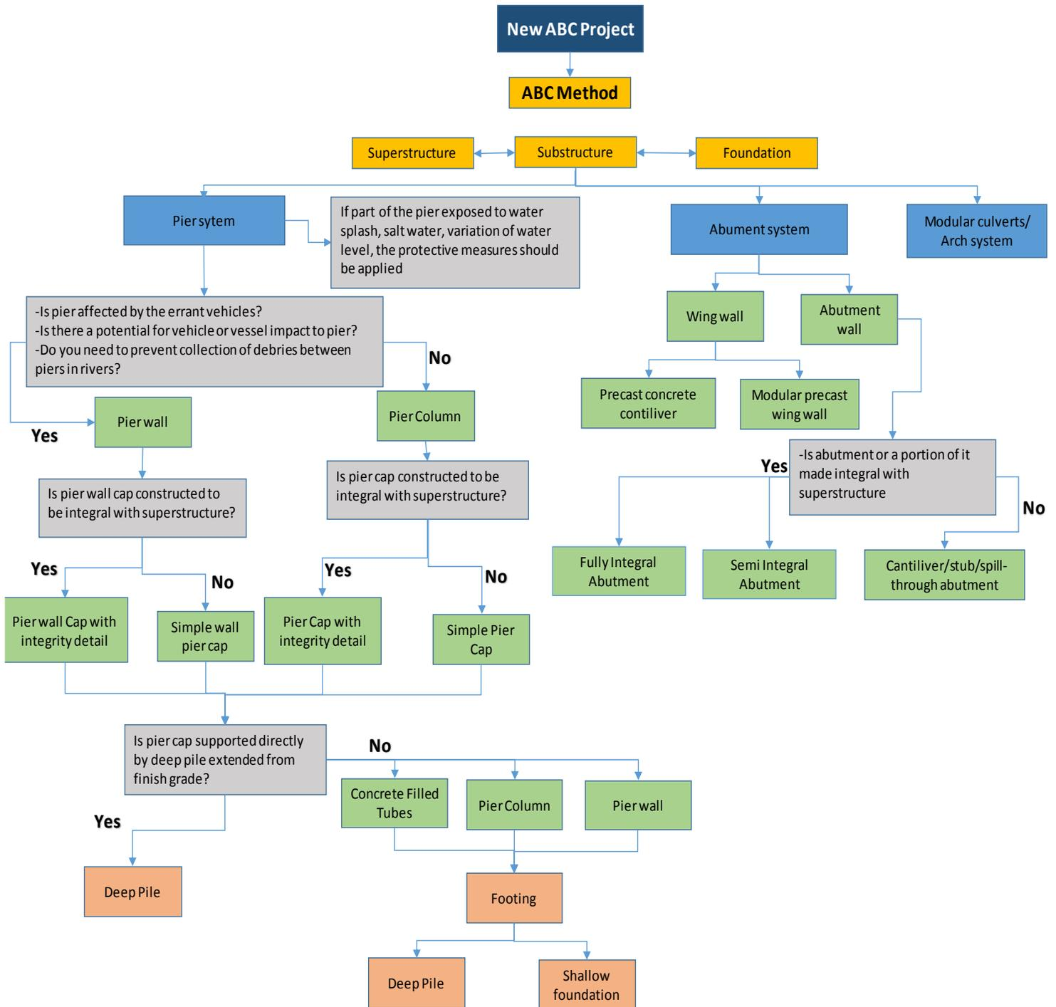
Figure 7: Preliminary flowchart for selection of substructures
