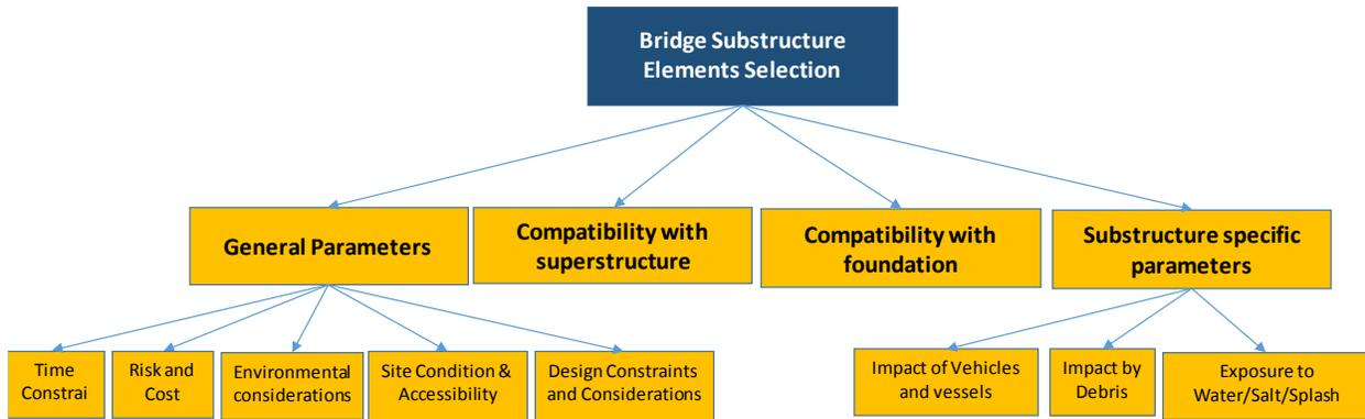
Figure 6: Bridge substructure element selection parameters
