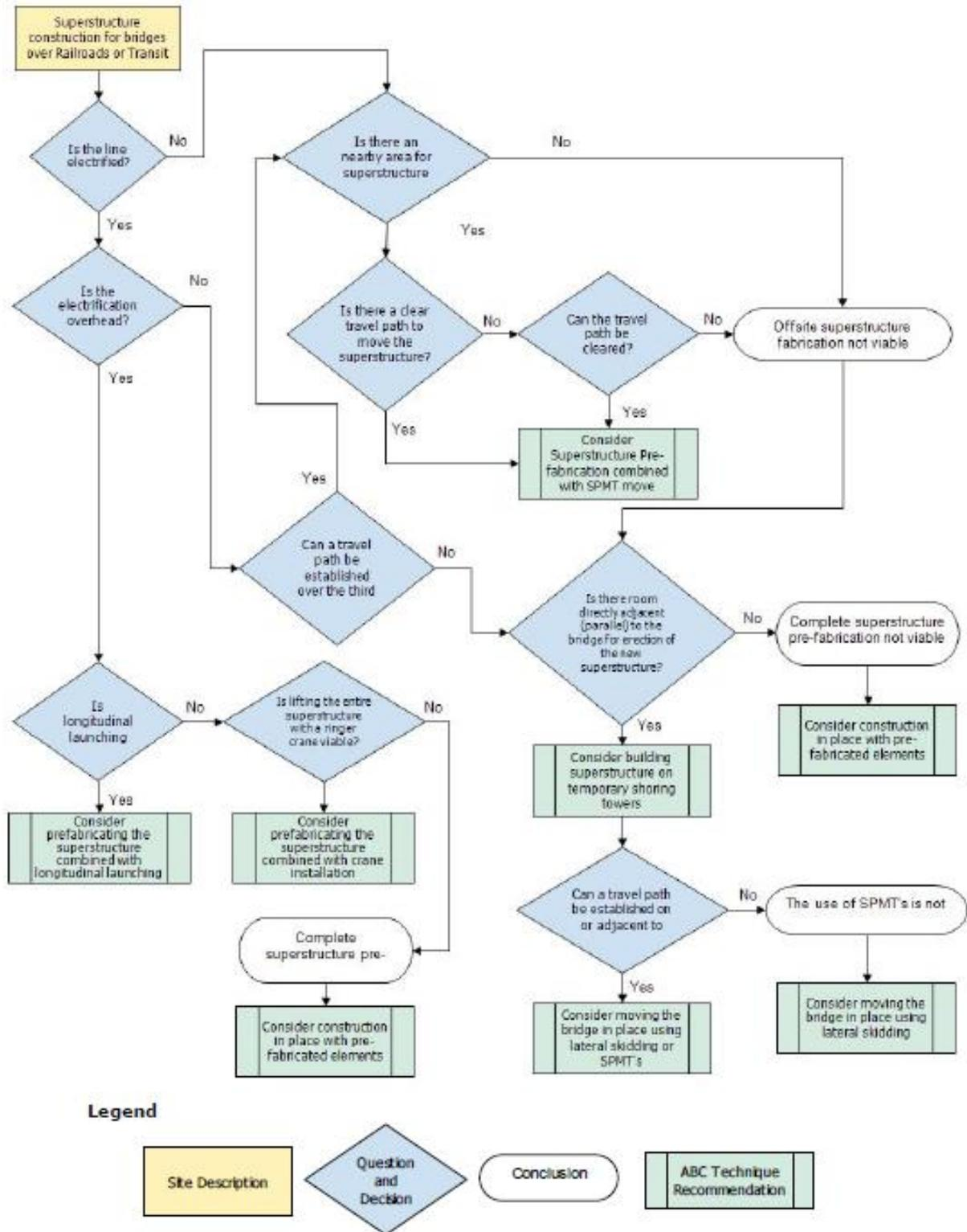
Figure 4: Decision flowchart for superstructure construction over the railroads [2]
