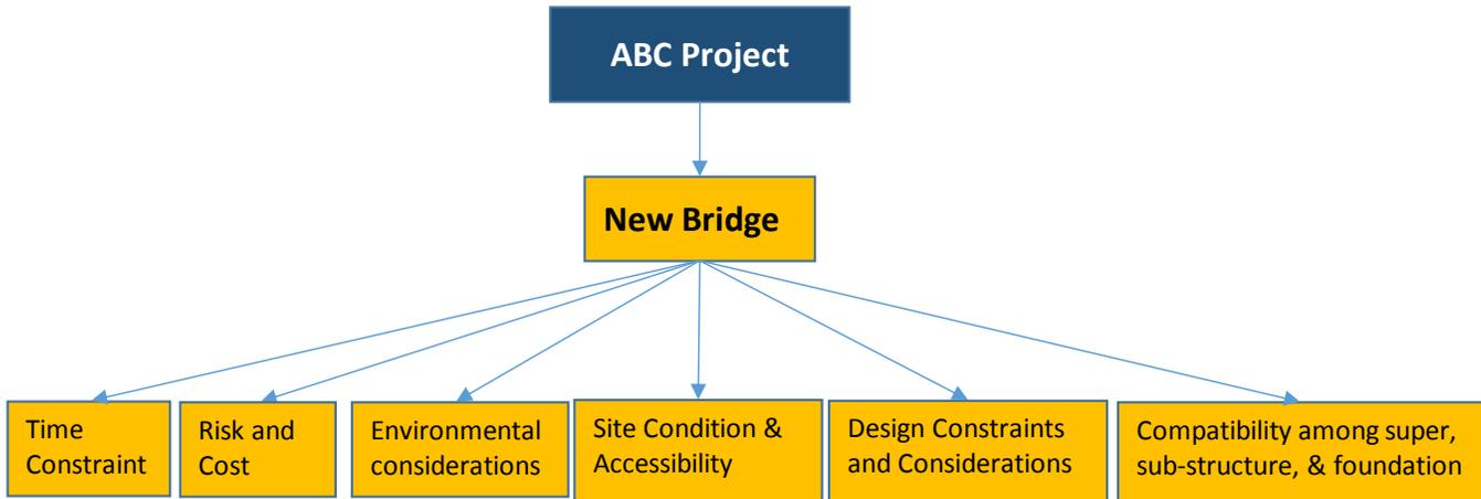
Figure 2: Parameters affecting selection of ABC components
