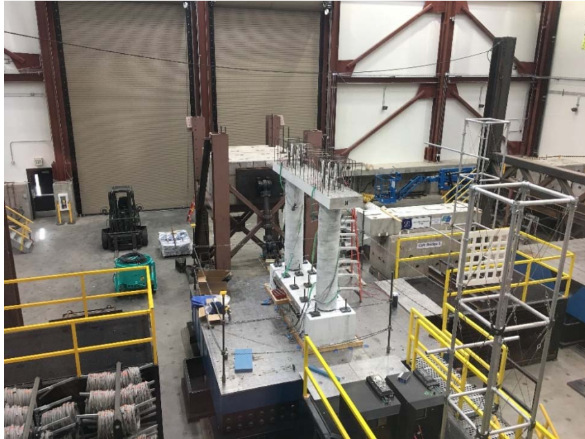
Fig. 60 – Two-column bent secured to the shake table
