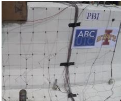
Figure 5.5. Test 1 (PBI middle) barrier cracks
