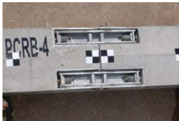
Figure 2.24. Side bolts and shear tube connection improvements
