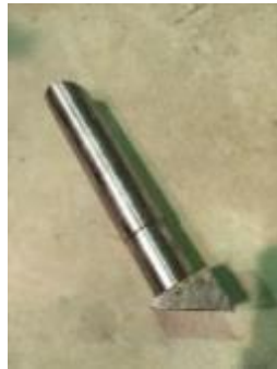
Figure 4.6. Inclined bar connection in deck
