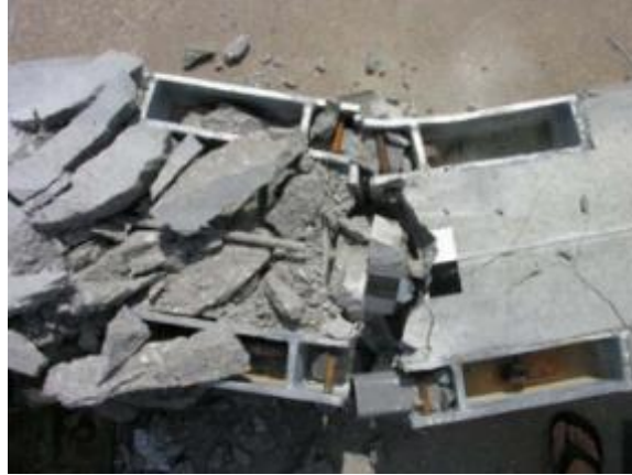
Figure 2.19. Side bolt and shear tube connection failure
