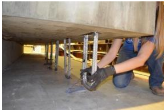
Figure 4.19. Insertion of U-bars
