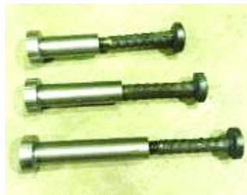
Figure 4.3. Transverse double-headed ties used for barrier-to-barrier connection
