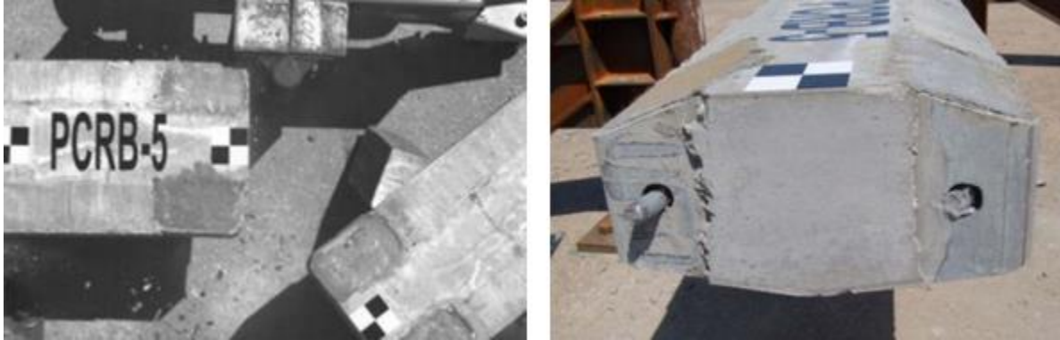
Figure 2.23. Alternate redesign I-shaped rail connection failure
