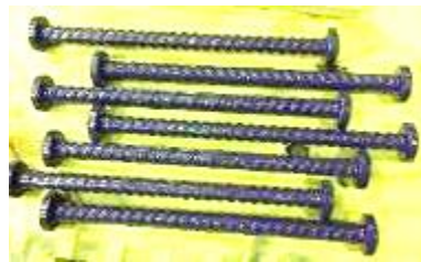
Figure 4.2. Longitudinal double-headed ties used for barrier-to-barrier connection
