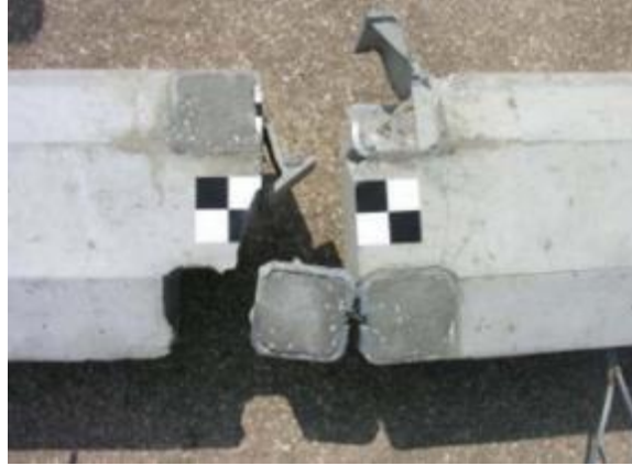
Figure 2.17. Failed MWRSF I-shaped rail connection
