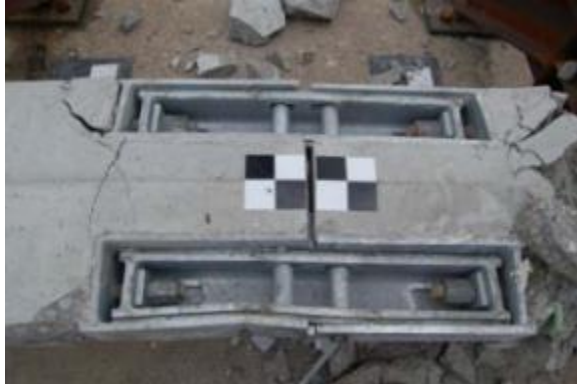
Figure 2.25. Side bolt and shear tube connection after testing
