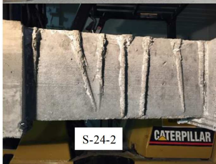
FIGURE 3 Detail of the test specimens surface before sand blasting.
