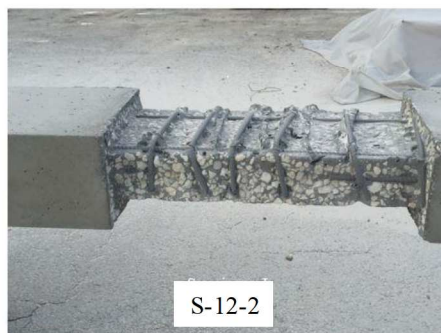
FIGURE 3 Detail of the test specimens surface before sand blasting.
