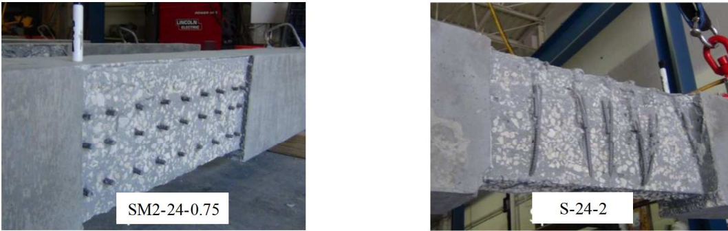
FIGURE 4 Detail test specimens surface after sand blasting.
