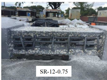
FIGURE 3 Detail of the test specimens surface before sand blasting.
