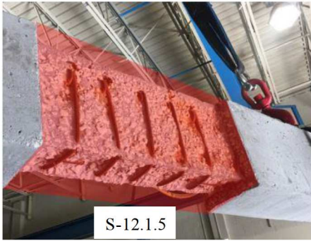
FIGURE 2 UHPC shell detail.
