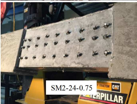
FIGURE 3 Detail of the test specimens surface before sand blasting.
