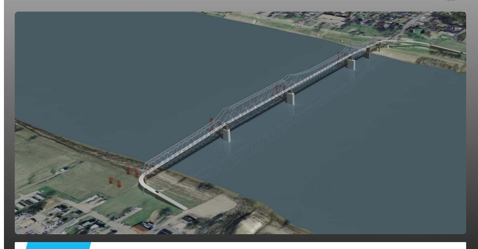
Downstream temporary support towers are constructed
