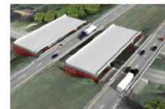
Step 1: Construct superstructure next to existing bridges
