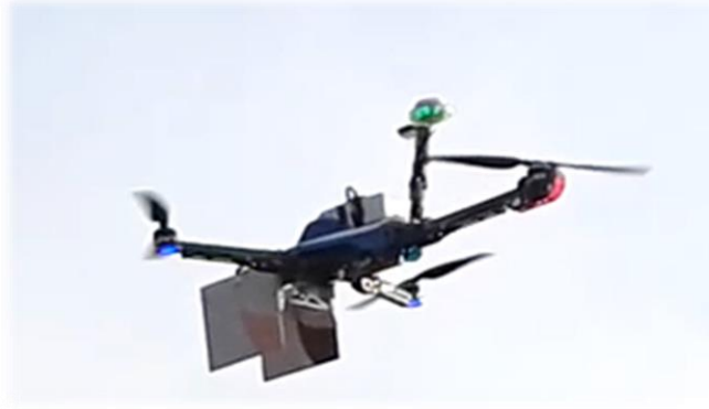
Figure 6. DAA GPR platform in action, including AVA antenna and synchronized IMU/GPS
