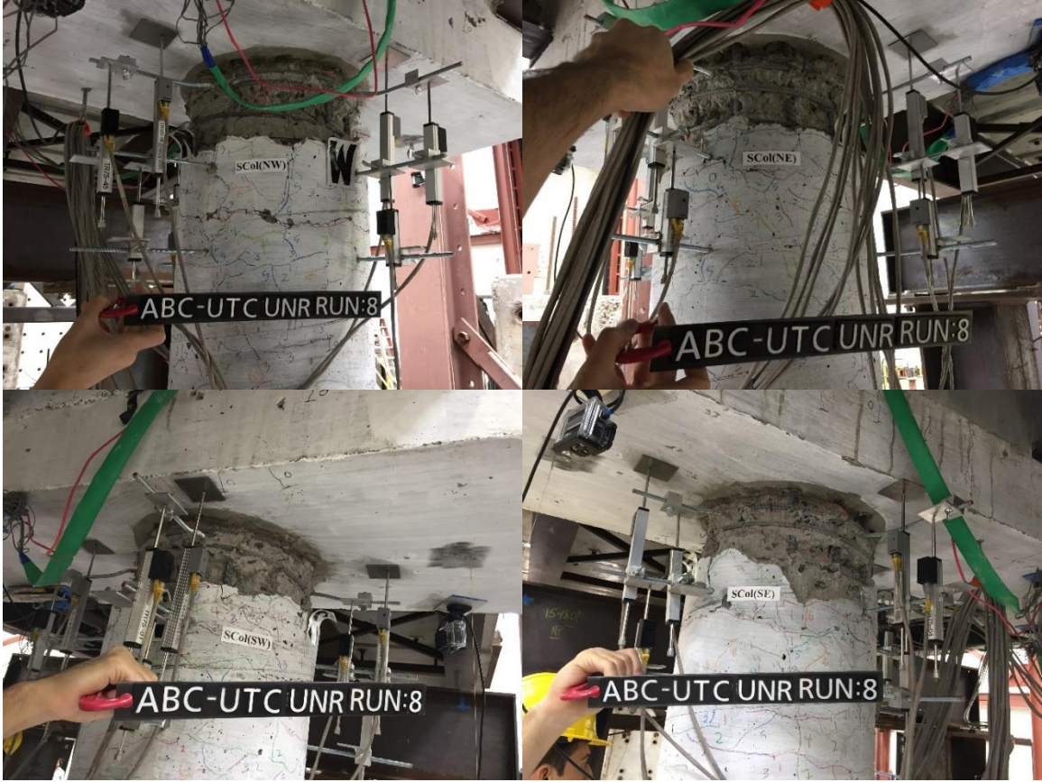
Figure B.9 Damage states of the south column plastic hinges after Run 8
