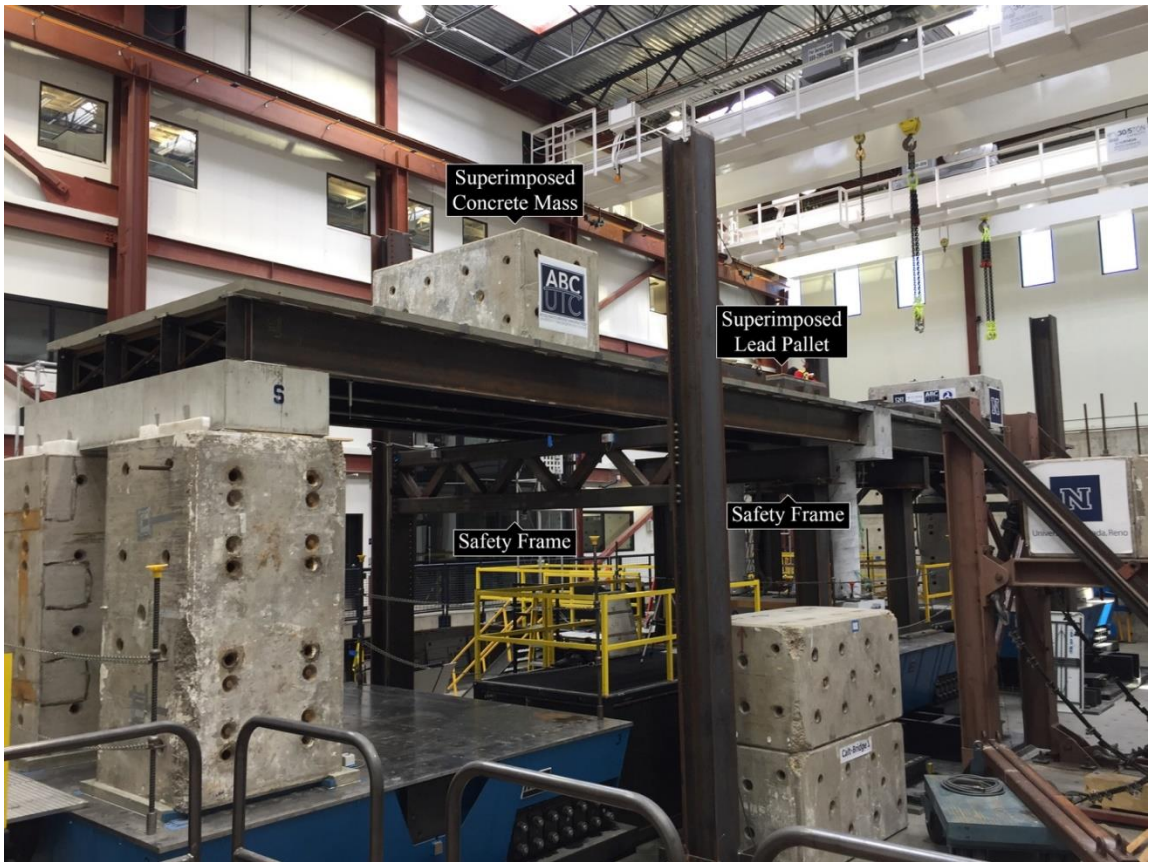
Figure 3.12 Test setup (Image by Elmira Shoushtari)
