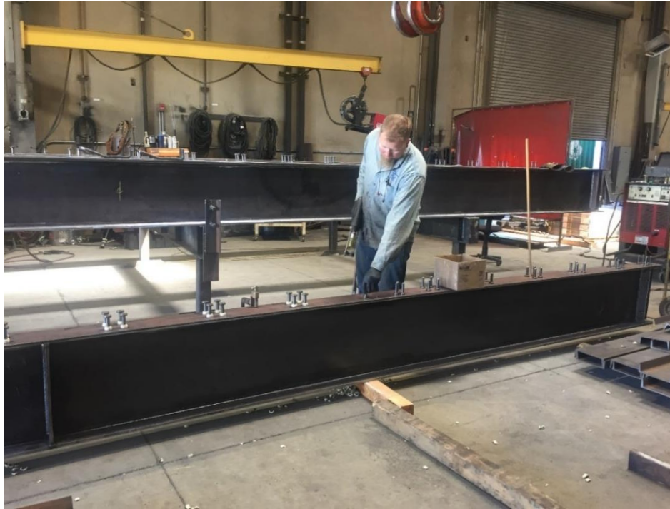
Figure A.23 Shooting the studs
