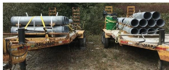
Figure 5 - Threaded N80 Casing in 5-ft Lengths
