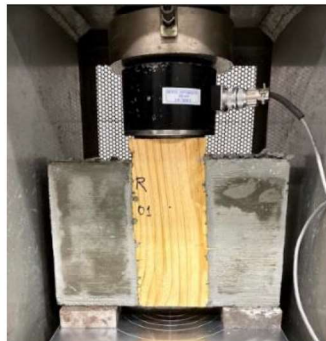
Figure 7. Push-off test setup.
