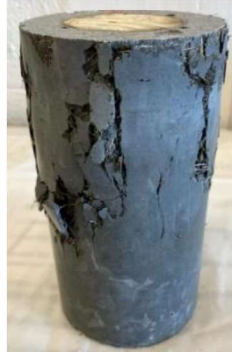
Figure 14. Failure mode of one of tested specimen
