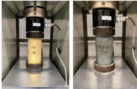
Figure 13. Test setup for load-carrying capacity. (a) timber specimen, (b) timber cylinder with UHPC encasement.
