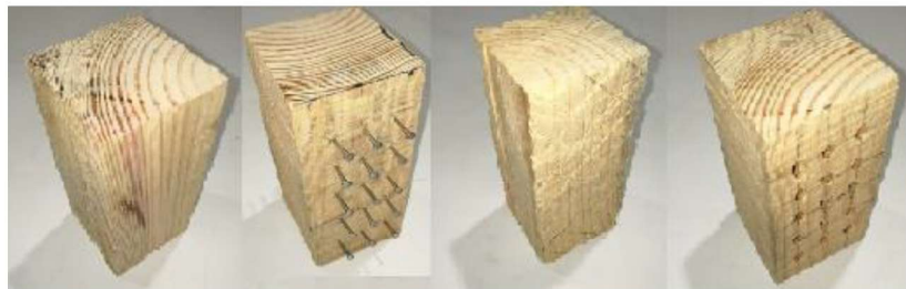
Figure 6. Different surface preparation for timber prisms
