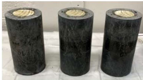
Figure 10. Sample for final timber cylinders with UHPC encasement.
