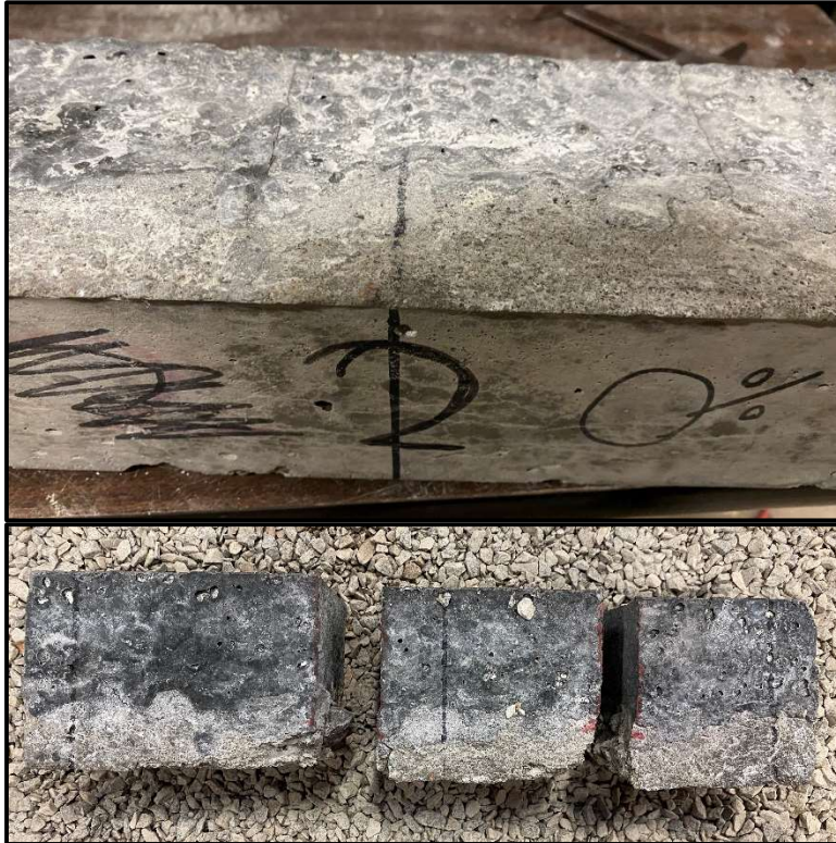
Figure 24. Splitting failure of composite freeze-thaw specimen with no steel fibers after 150 cycles (top) and after 350 cycles (bottom)
