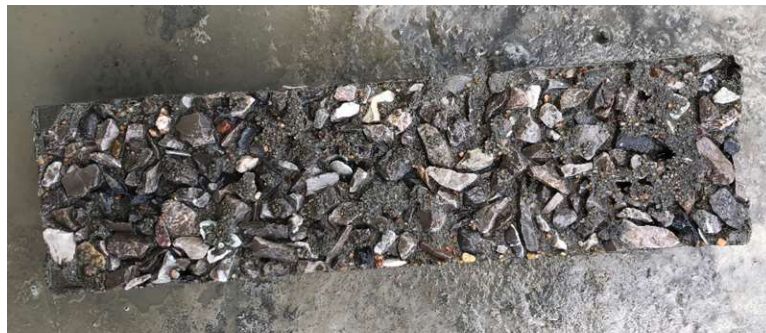
Figure 21. Exposed aggregate surface of base concrete used for composite freeze-thaw specimen
