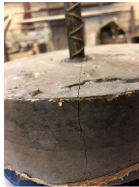
Figure 15. Splitting failure of preliminary pullout specimen with 2d_b embedment
