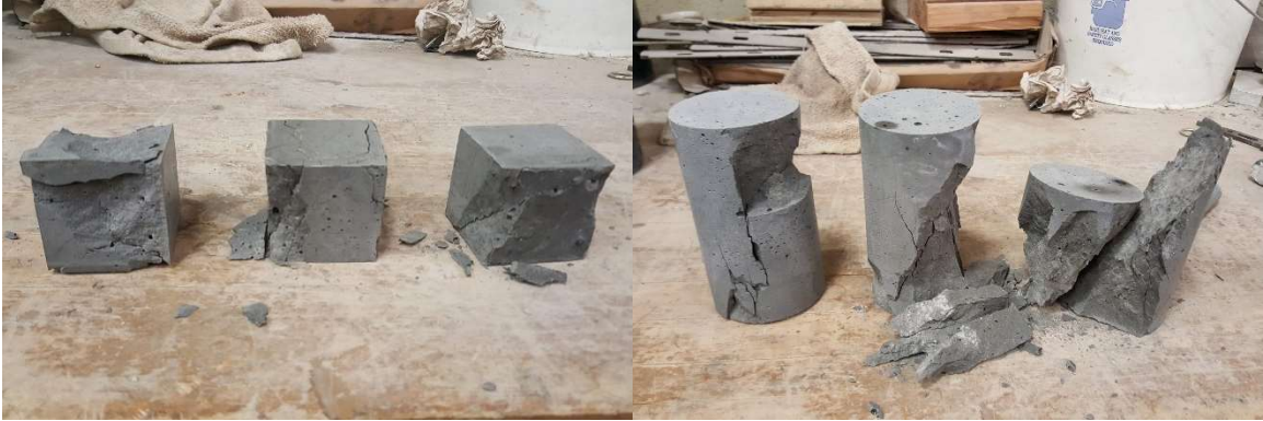
Figure 3. Example tested compressive strength specimens (0% fiber mix)
