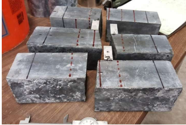
Figure 6. Example tested modulus of rupture beam specimens (0% fiber mix)
