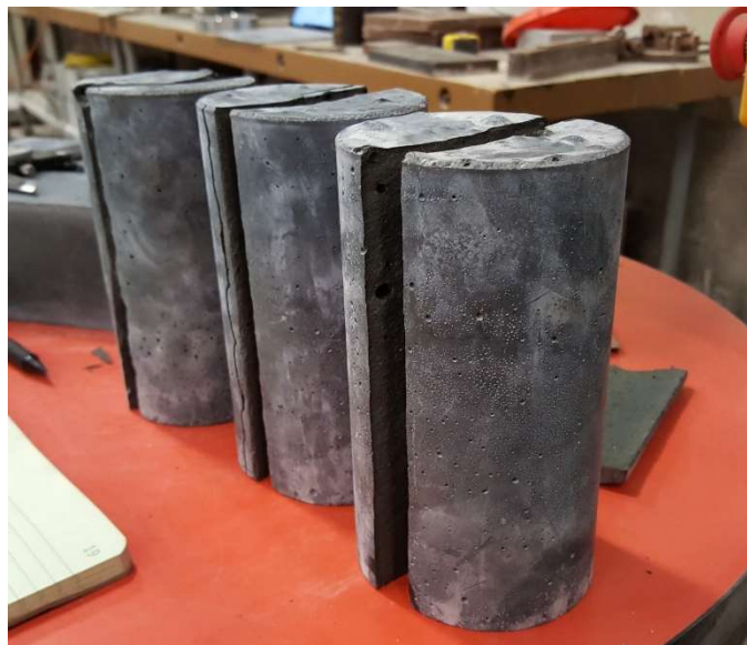
Figure 5. Example tested splitting tensile strength specimens (0% fiber mix)
