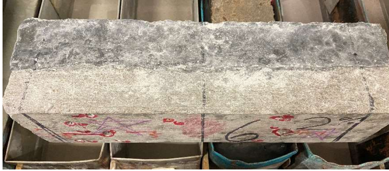
Figure 22. Composite freeze-thaw specimen
