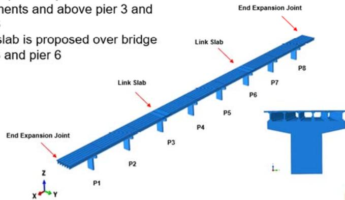
Figure 5 Finite-element model of the case study bridge
