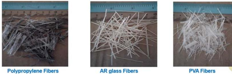
**Figure 3 FRC developed in the ISU for link slab applications**
