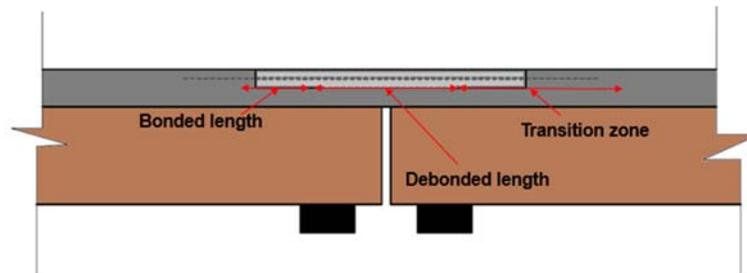
Figure 2 Link slabs and different parts of link slab shown in a slide
