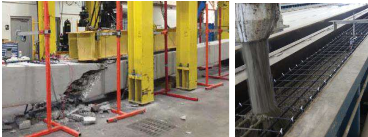
Figure 10: Flexural testing of PPCP with CFCC (Roddenberry et al., 2014)
