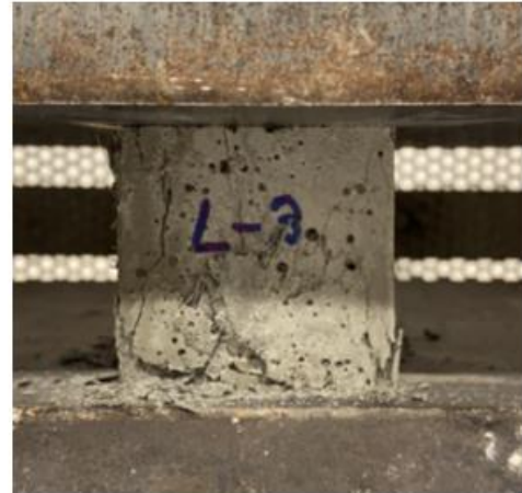
Compression test of cubes
