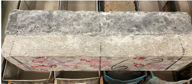
Figure 22. Composite freeze-thaw specimen
