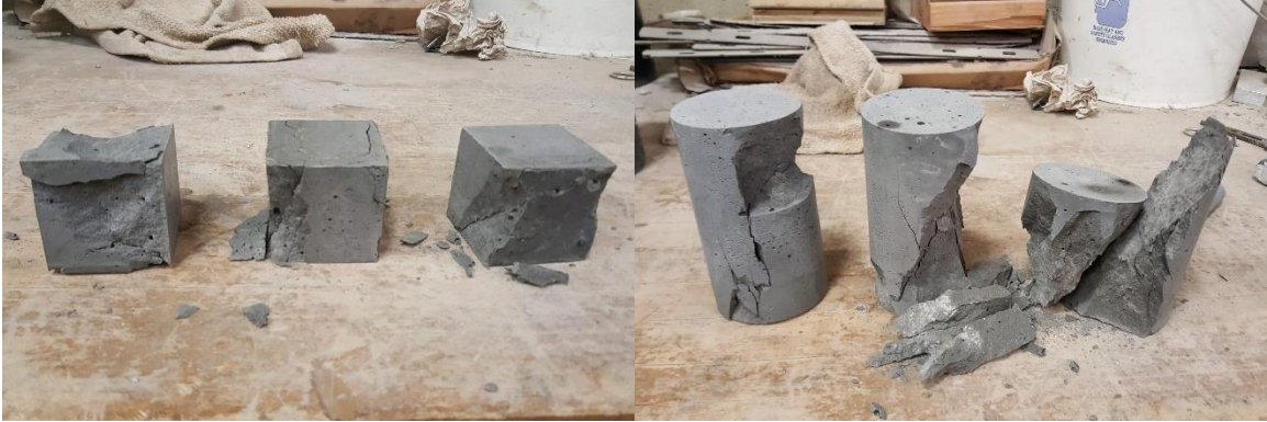
Figure 3. Example tested compressive strength specimens (0% fiber mix)
