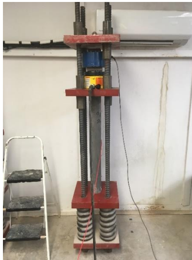
Figure 7. Example creep specimen immediately after loading (0% fiber mix)
