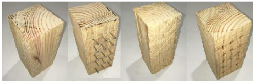
Figure 6. Different surface preparation for timber prisms
