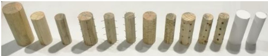
Figure 12. Different surface preparation for timber prisms
