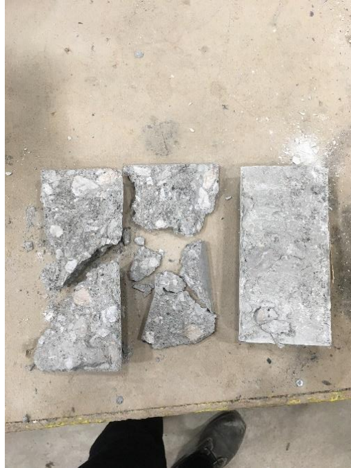
Figure 5.27. Cylinder 3 split cylinder failure
