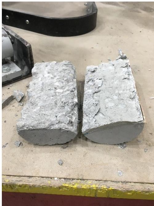
Figure 5.26. Cylinder 2 split cylinder failure
