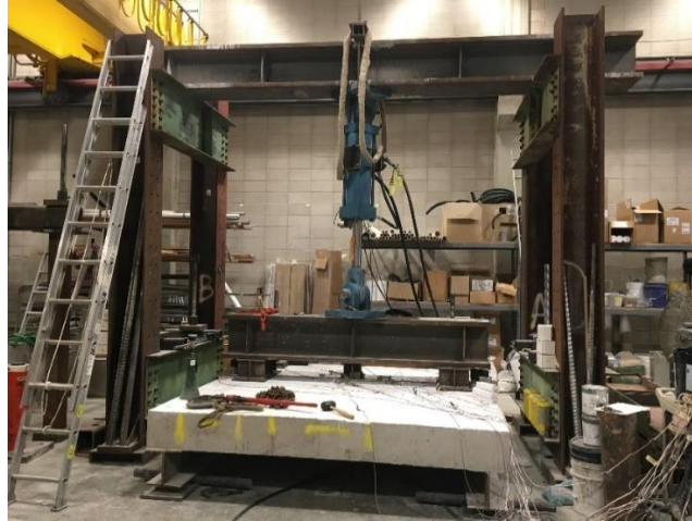
Figure 5.32. Fatigue loading setup
