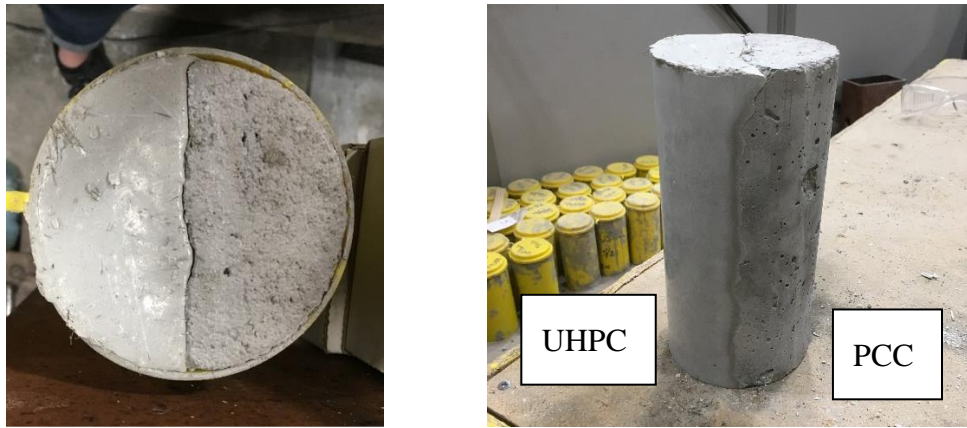
Figure 5.23. Split cylinder interface
