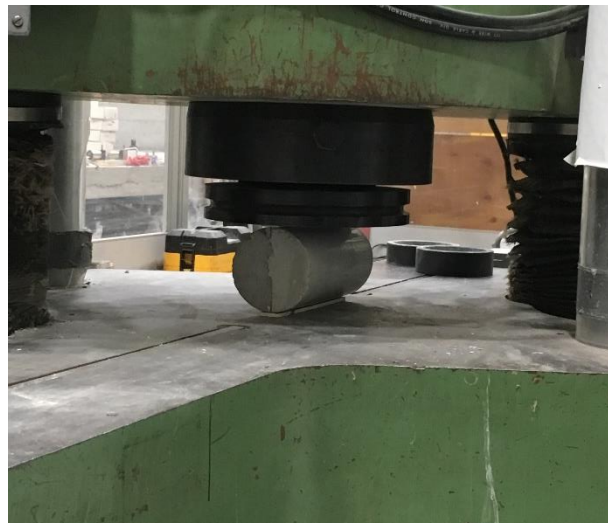
Figure 5.24. Split cylinder test
