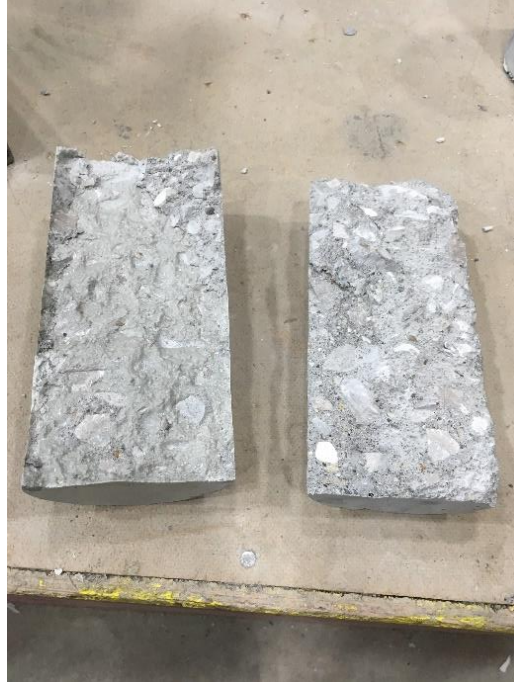
Figure 5.25. Cylinder 1 split cylinder failure
