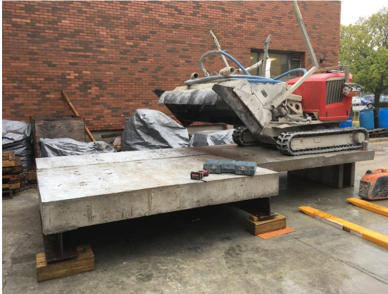
Figure 5.13. Aquajet aqua cutter 710H
