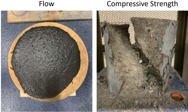
Variables that have been evaluated are: water-to-cement ratio, binder-to-aggregate ratio, binder proportions (cement, slag, silica fume), cement type, super plasticizer content, viscosity modifying admixture content, mixing procedure and time at which admixtures are added, moisture content of fine aggregates, steel fiber type and quantity, and curing type. Best results from these mixes have been between 15 and 20 ksi at 28 days.
