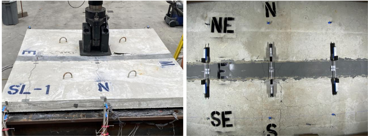
Figure 26 – Damage scheme of specimen S4.
