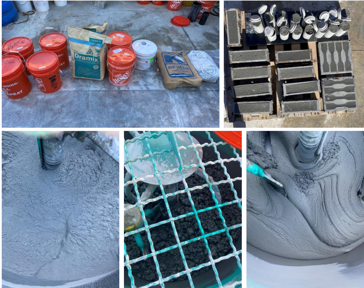
Figure 9 – Non-proprietary UHPC mixing of trial mix “B2-NV-2%-S” at UNR.
