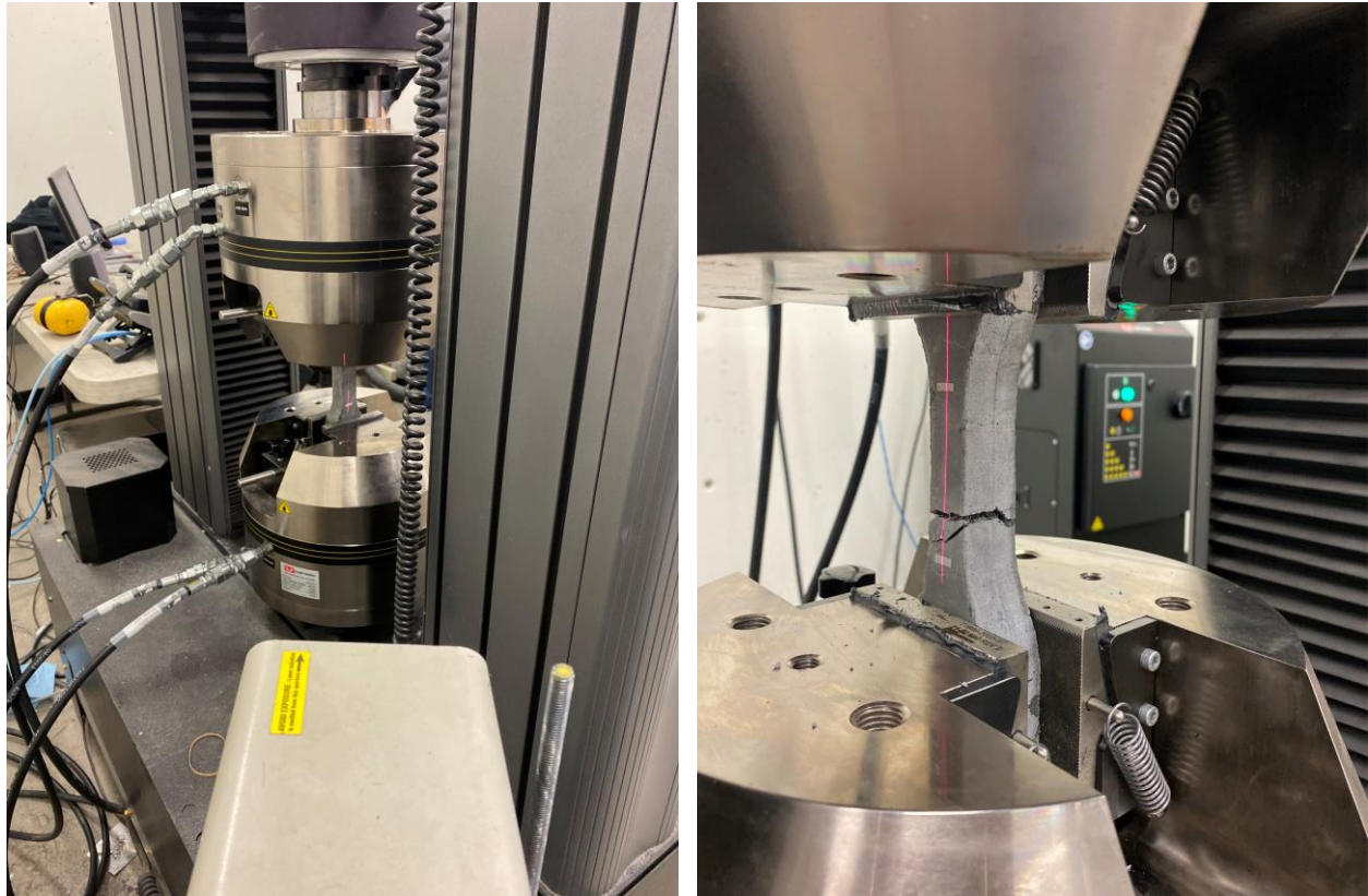
Figure 15 – tension tests of the non-proprietary UHPC dog-bone samples at UNR.
