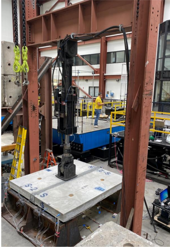
Figure 16 – Test setup for transverse specimens.
