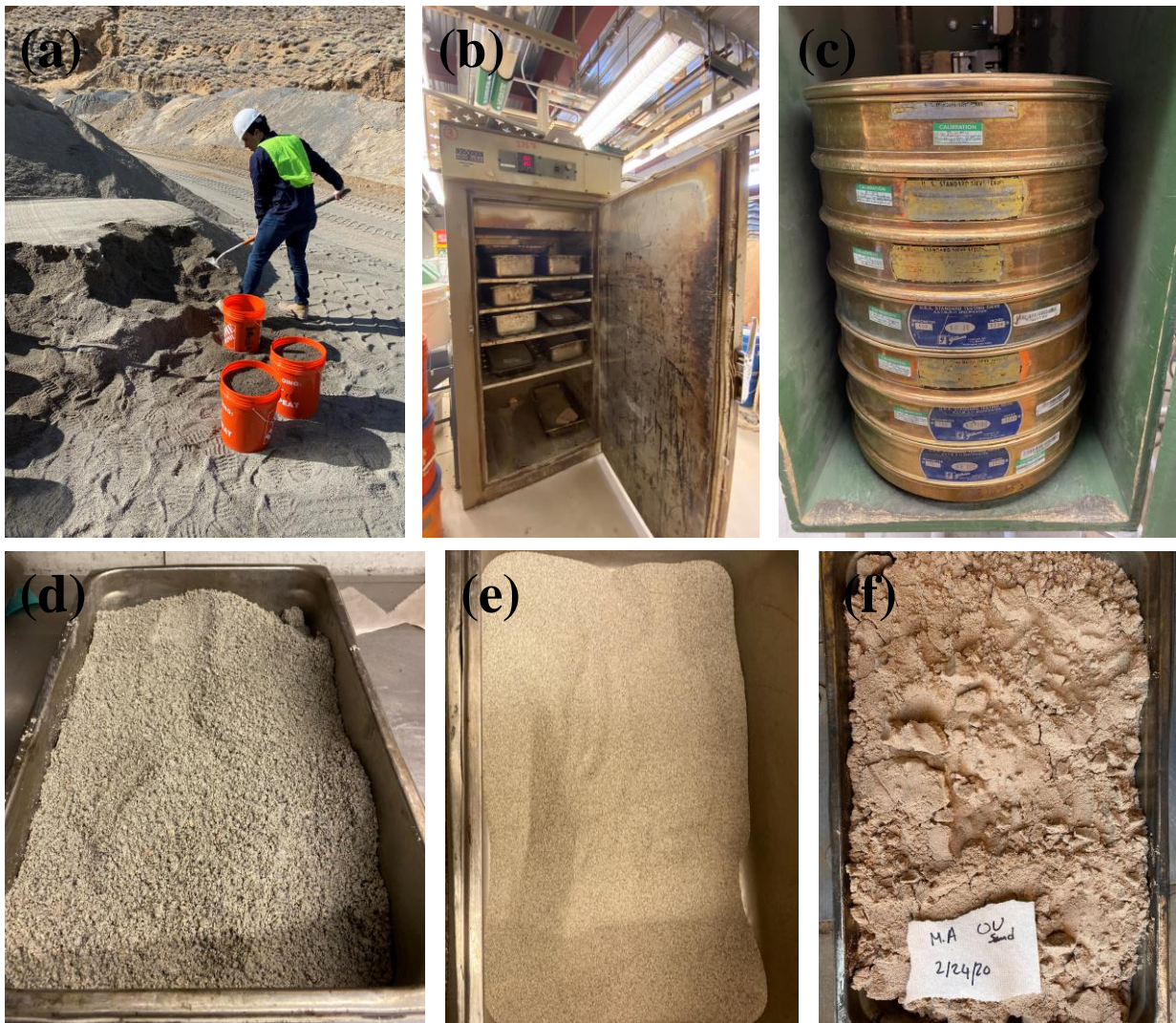
Figure 8 – (a) packing of the crushed aggregate sand, (b) sand drying, (c) sand sieving, (d) crushed aggregate sand without sieving, (e) Crushed aggregate sand after sieving, and (f) OU sand.
