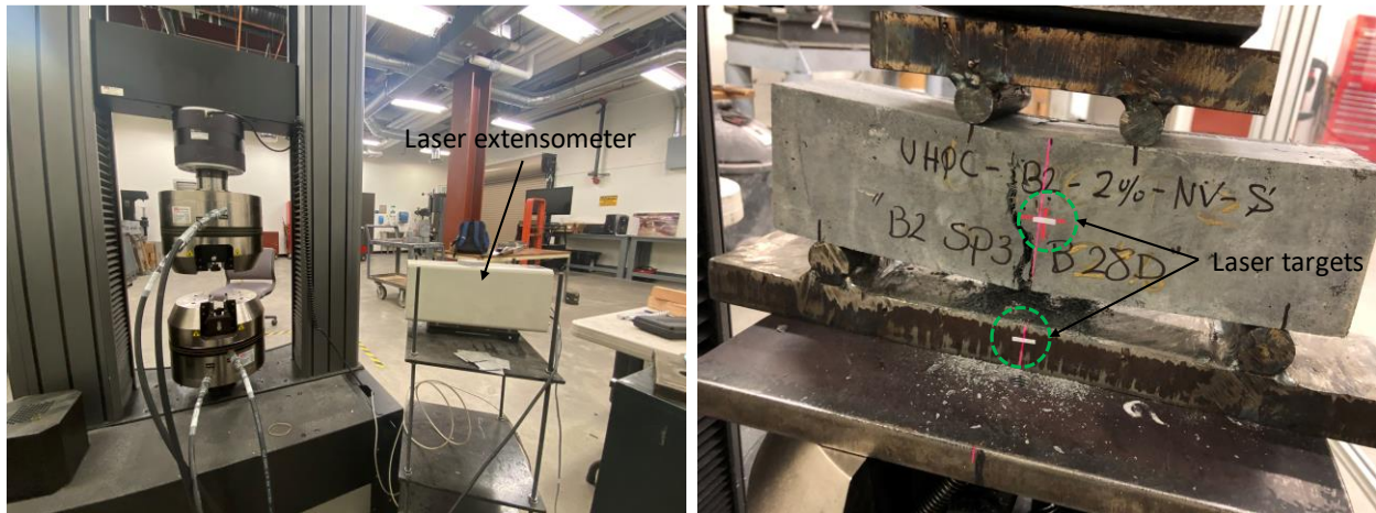
Figure 14 – Bending tests of the non-proprietary UHPC beams with using the laser extensometer at UNR.
