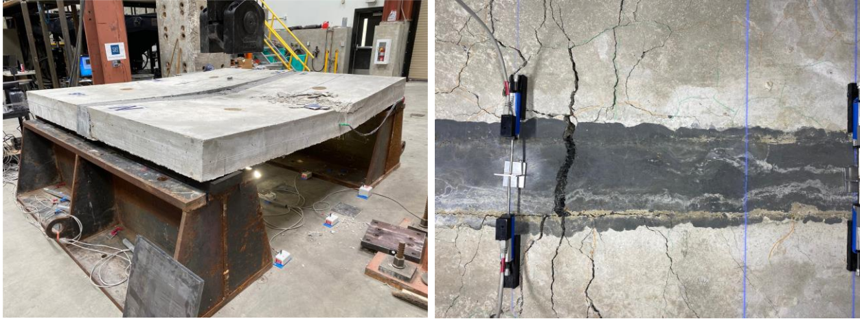
Figure 23 – Damage scheme of specimen S1.
