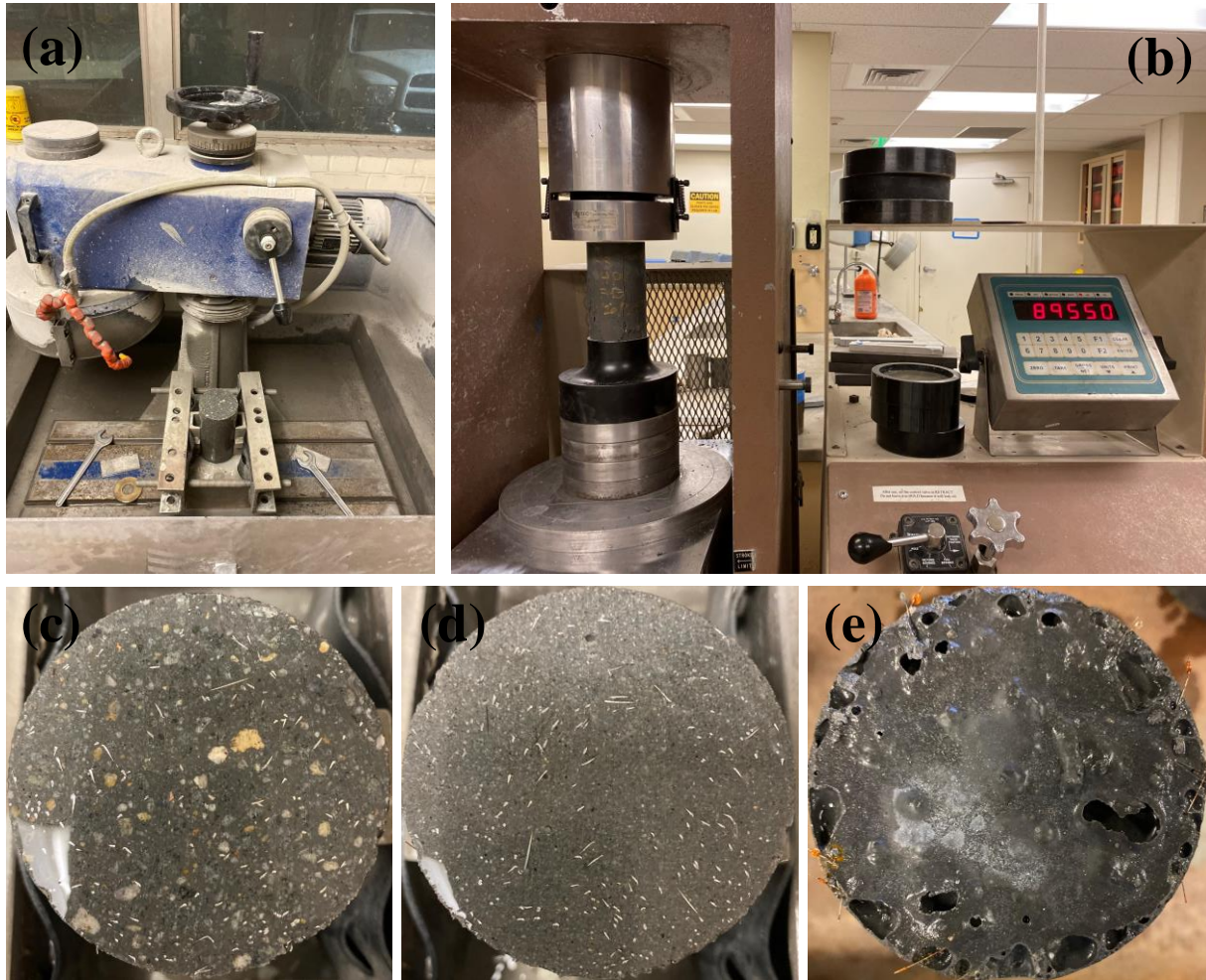
Figure 11 – (a) Grinding machine at UNR, (b) Satic compression machine at UNR, (c) UHPC cylinder from B3 after surface grinding, (d) UHPC cylinder from B4 after surface grinding, and (e) UHPC cylinder with air voids at the top part before saw cutting and grinding.
