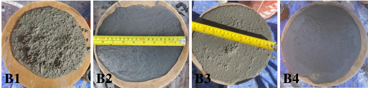
Figure 10 – Flow tests of the trial Non-proprietary UHPC mixes at UNR.
