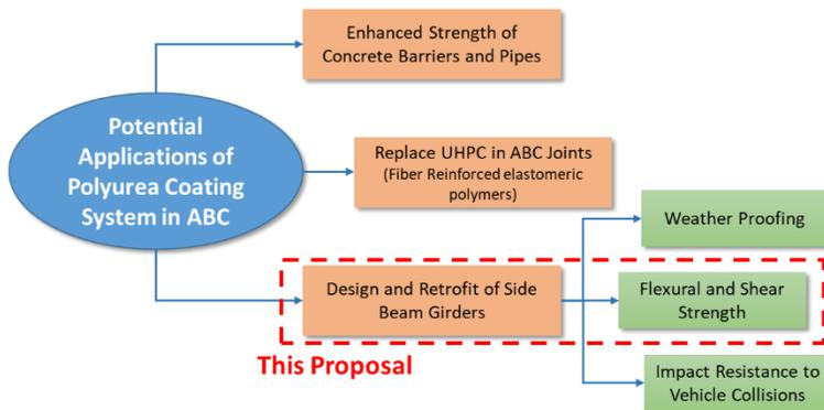
Figure 2: Potential applications of the polyurea system in accelerated bridge construction. This proposal takes the first step of a long-term research vision to examine and investigate the innovative application of polyurea coating system.
