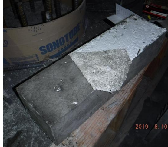
Figure 13. Flexural beam removed from form; roughness profile skin partially removed.
