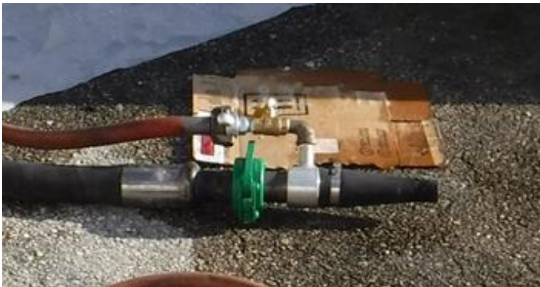
Figure 28. Nozzle with Air and Concrete lines connected.
