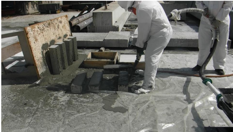
Figure 31. Application vertically down on flexure beam samples
