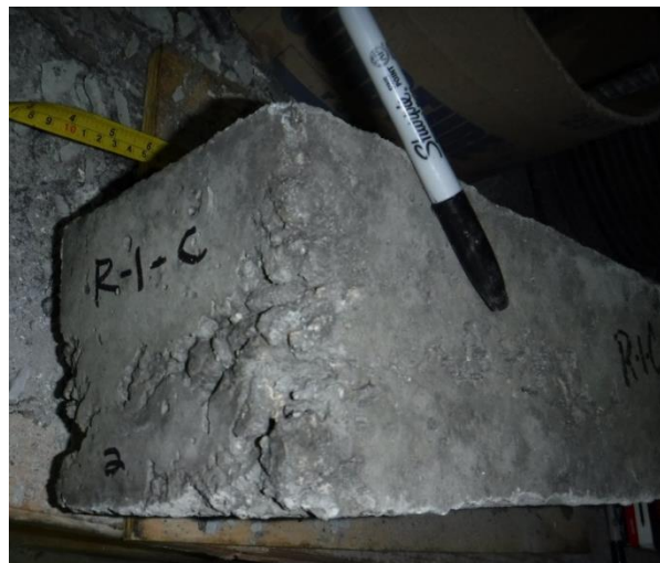
Figure 15. Flexural Beam R-1-C honeycombs
