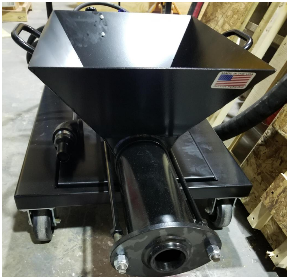
Figure 26. Black-Jack pump showing hopper and discharge.
