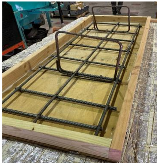
Figure 22. UHPC panel for bond testing and overlay testing of UHPC shotcrete.
