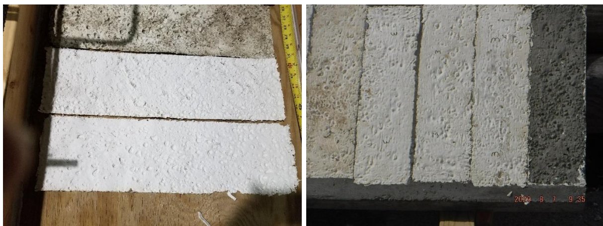
Figure 22. UHPC panel for bond testing and overlay testing of UHPC shotcrete.
