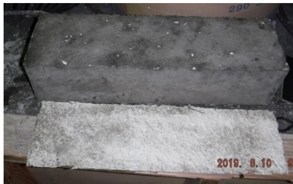
Figure 14. Flexural beam removed from form; roughness profile skin removed.
