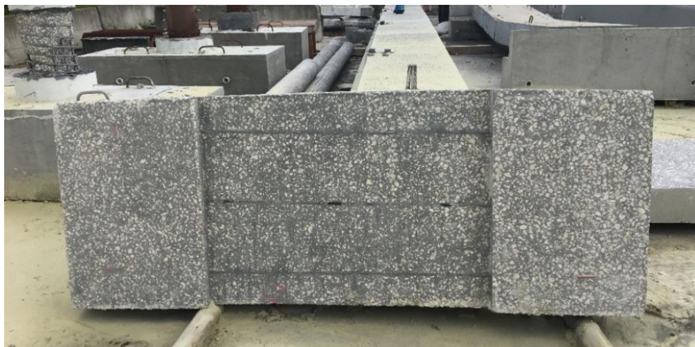
Figure 21. Sand-blasted slab specimen (Bottom-surface)
