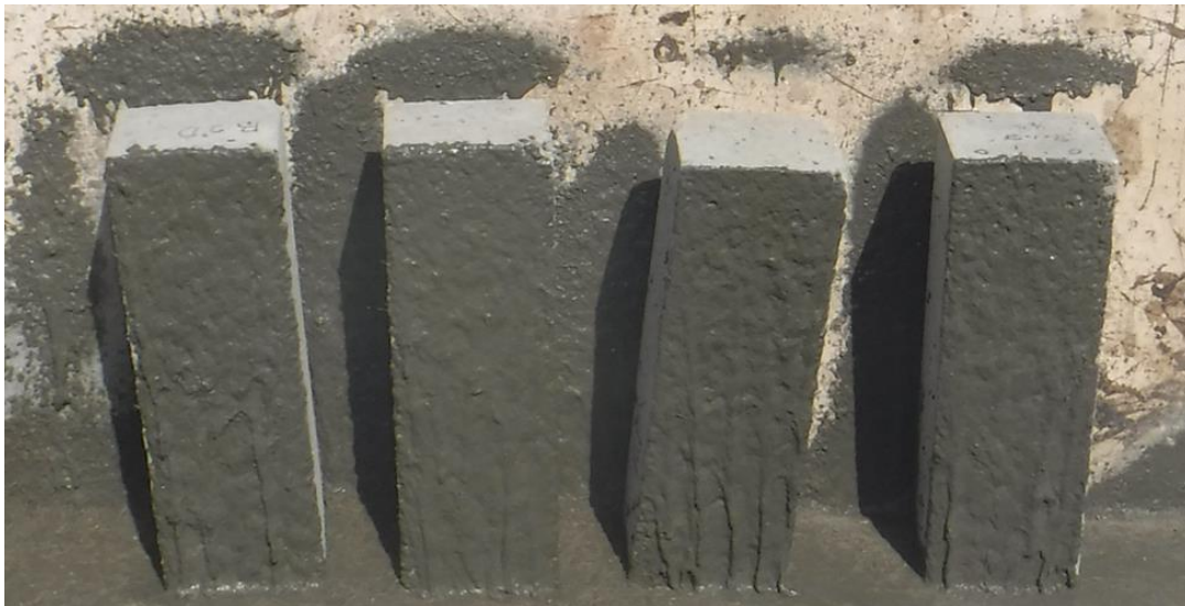
Figure 34. Horizontal application on flexural beam samples
