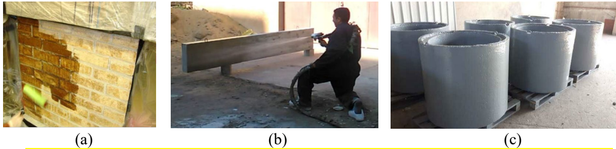
Figure 1: Application of polyurea coating (a) masonry slab (photo is taken from [4]), (b) RC beam specimens (photo is taken from [3]), and (c) concrete pipe (photo is taken from [5]).
