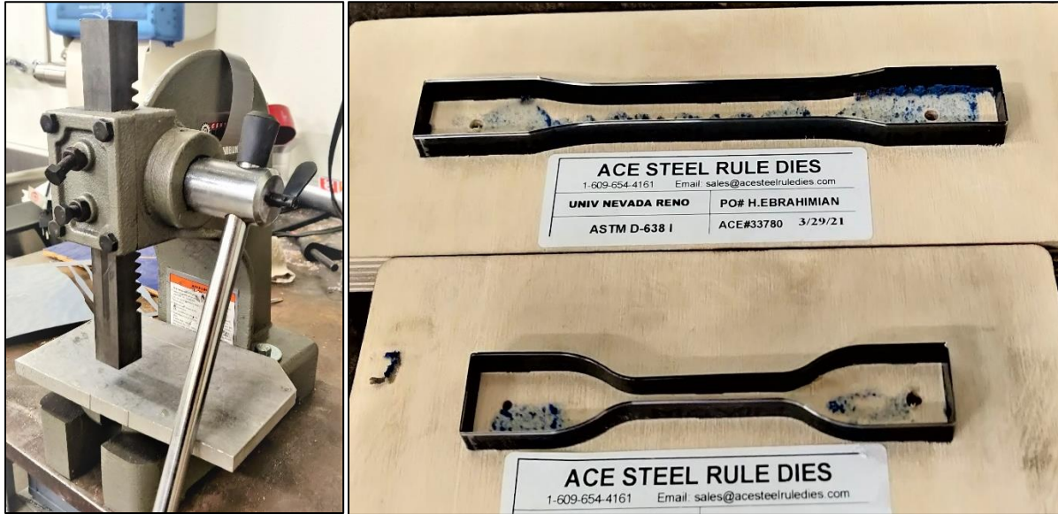
Figure A 1: (a) Arbor press (left) (b) ASTM Standard Die 1 (top) and Die 4 (bottom)
