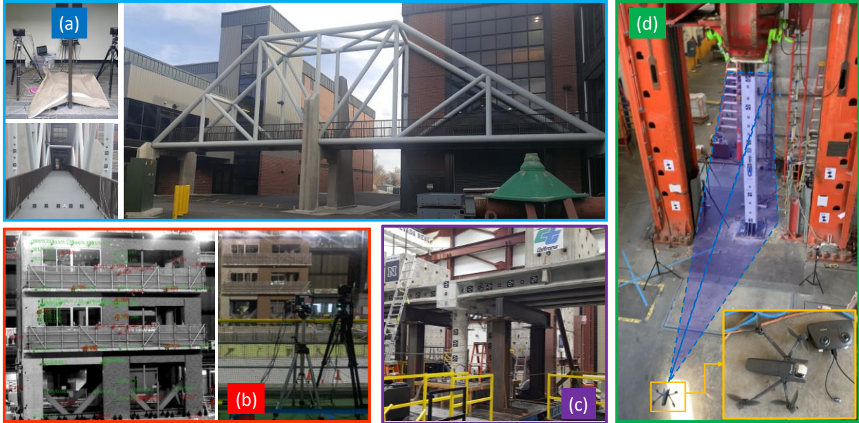
Fig. 1 Sample of vision-based monitoring of large-scale seismic tests and SHM field applications
