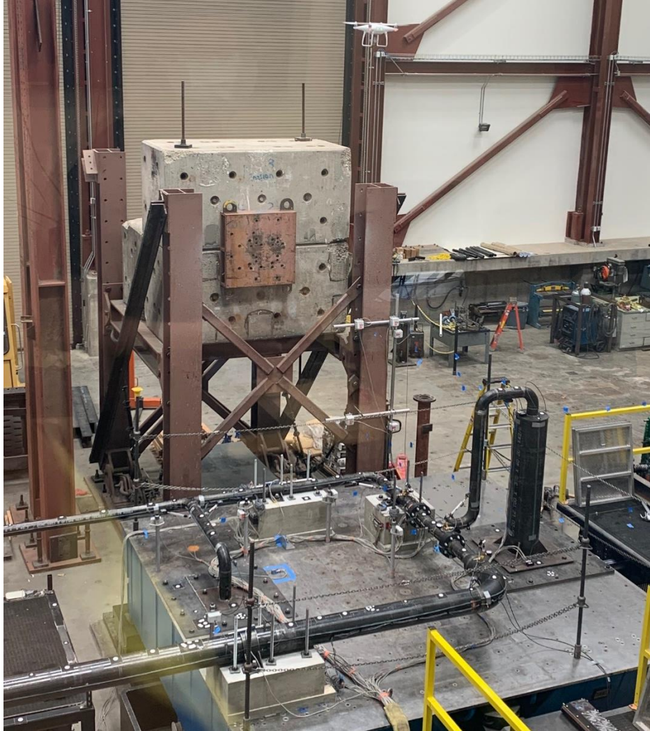
Fig. 3 – Example of a large-scale drone-based dynamic response monitoring of an infrastructure system tested at multiple shake tables at UNR.
