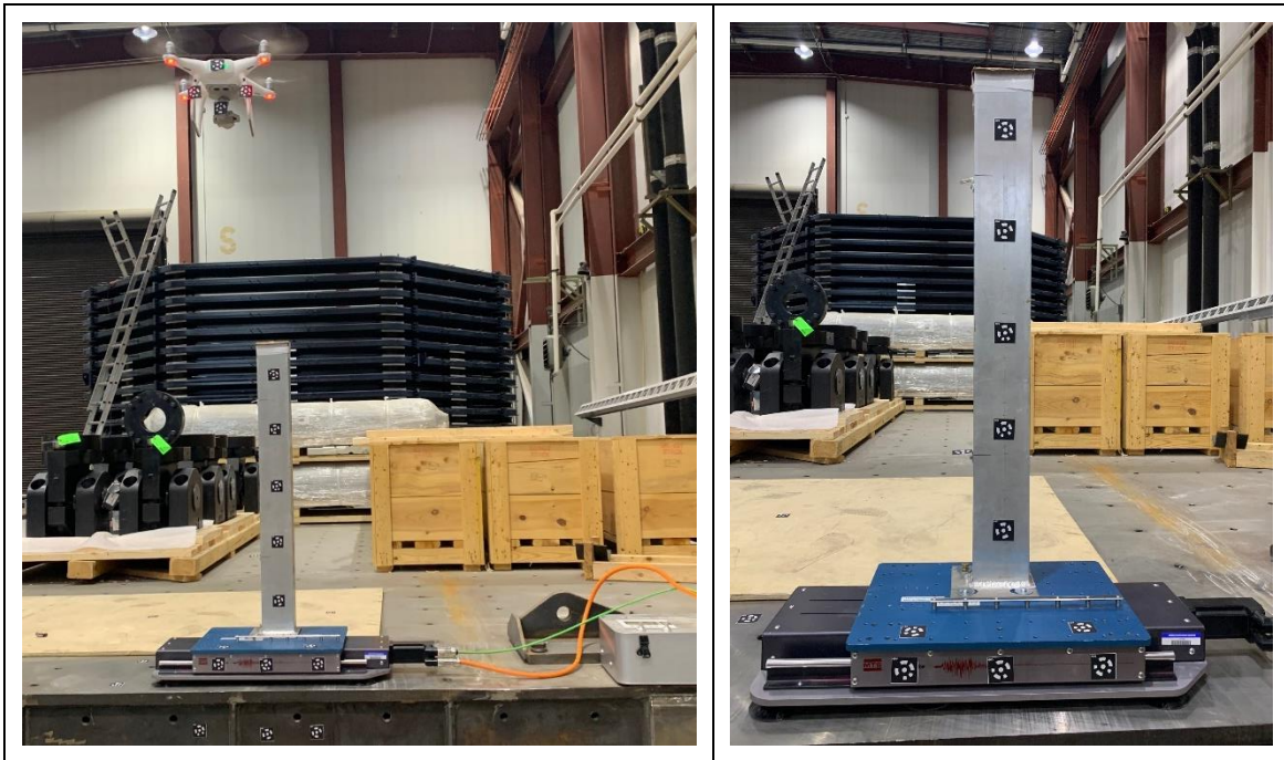
Fig. 2 – Example of a V&V test for drone-based dynamic response monitoring.
