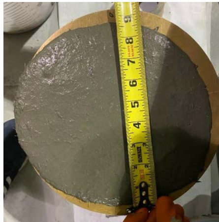
Figure 2: Workability of the material using flowability test (ASTM C1437)
