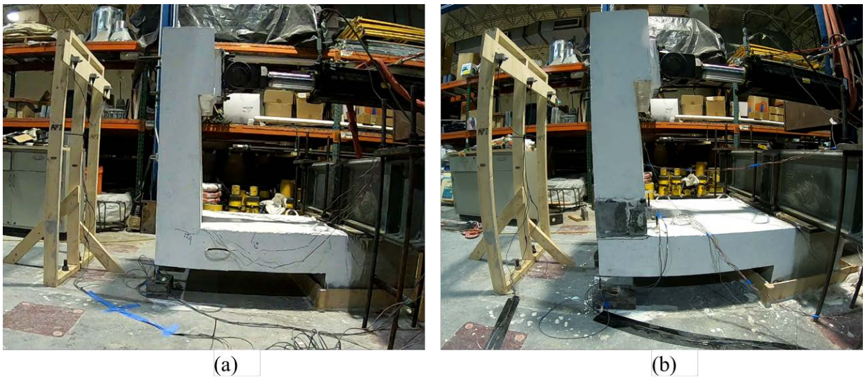
Figure 9- Load test setup for a) cast-in-place barrier and b) prefabricated barrier with UHPC connection.
