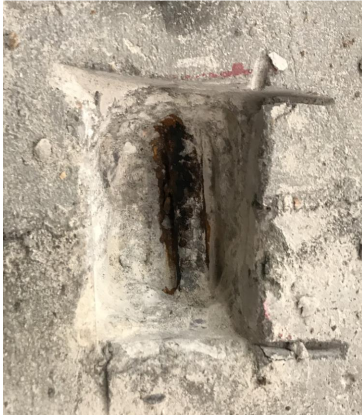
Class AA composite specimen post-corrosion testing: cut-out pocket at interface
