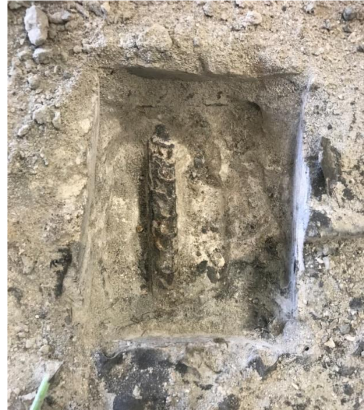
J3 non-proprietary UHPC composite specimen post-corrosion testing: cut-out pocket at interface
