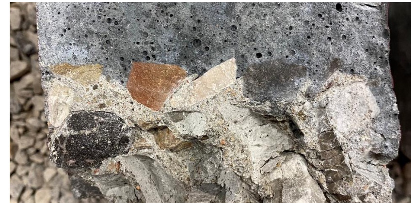
Close-up showing no damage at interface after freeze-thaw testing
