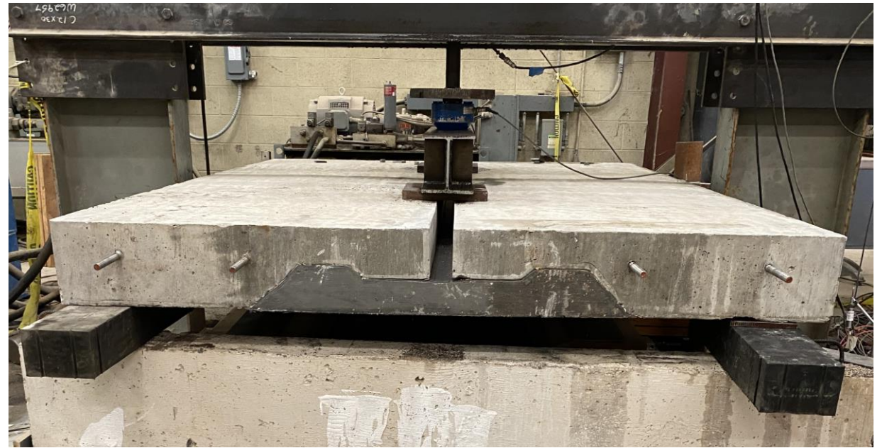
J3 non-proprietary UHPC link slab in tension loading (upside down of service orientation)
