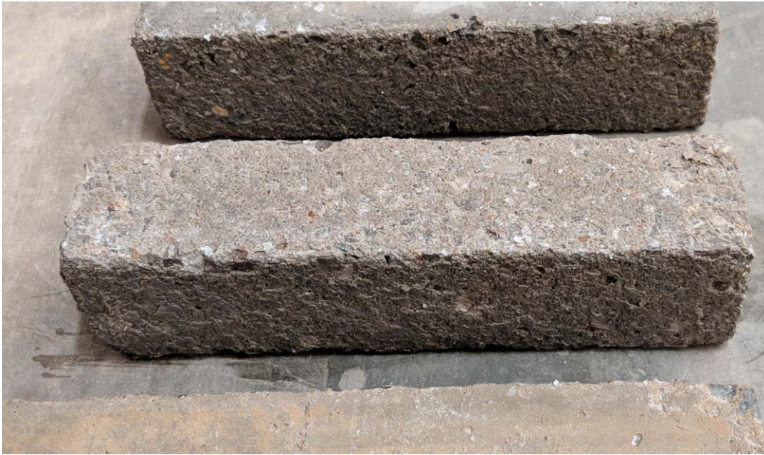
Class AA specimen section after freeze-thaw testing
