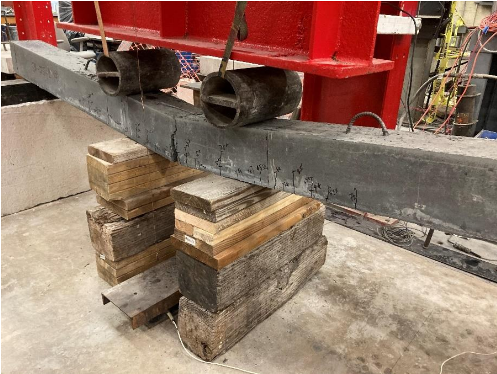
J3 non-proprietary UHPC specimen showing distributed cracking at failure
