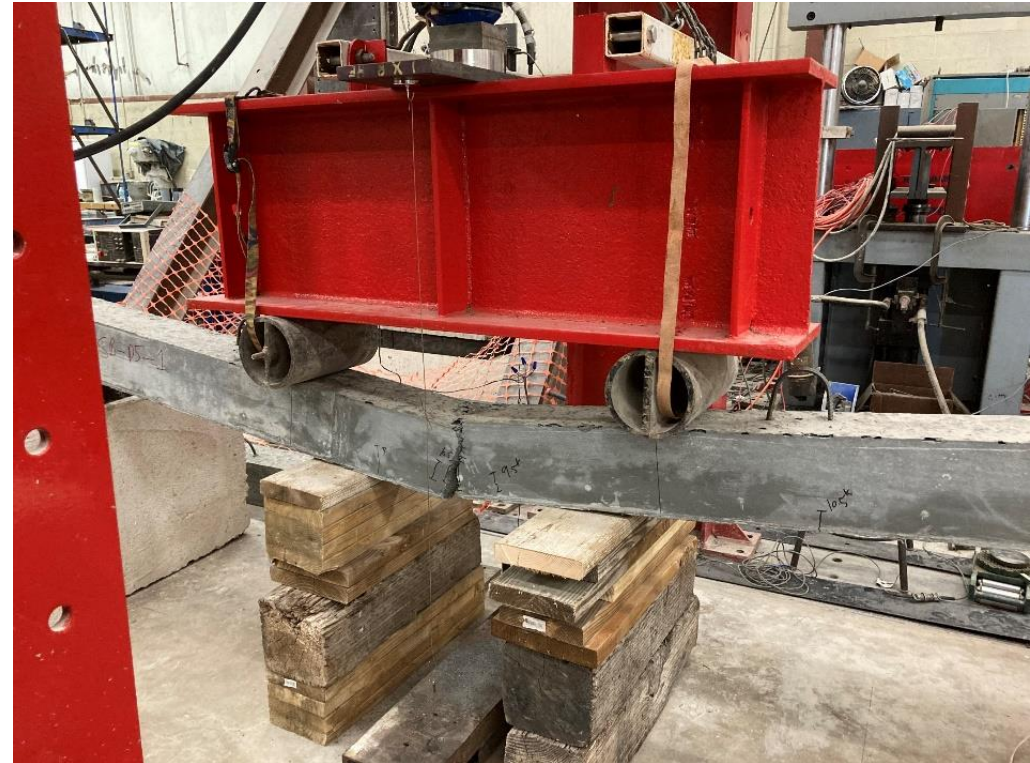
Proprietary UHPC specimen showing limited cracking at failure
