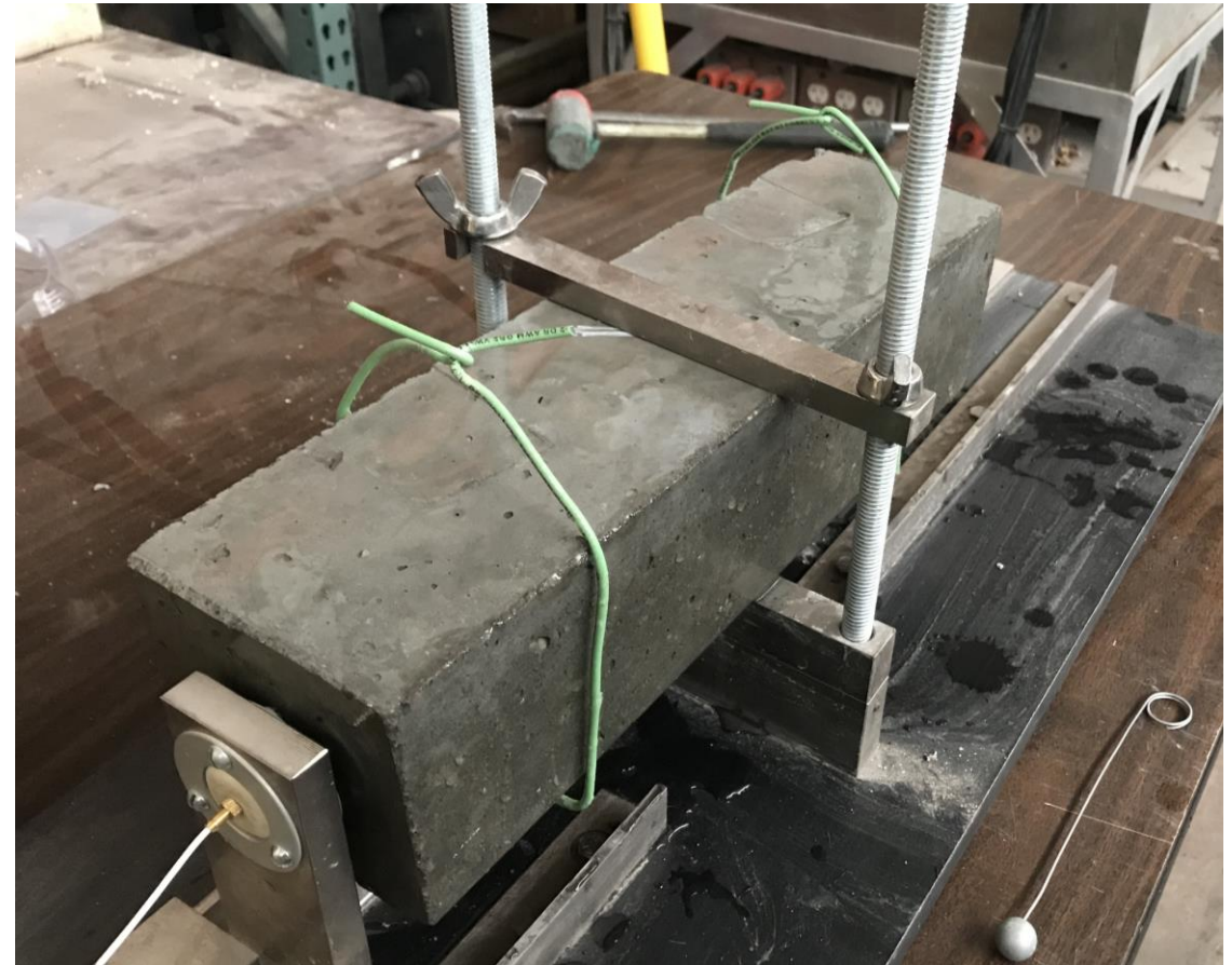
UHPC specimen set up for determining its fundamental transverse frequency
