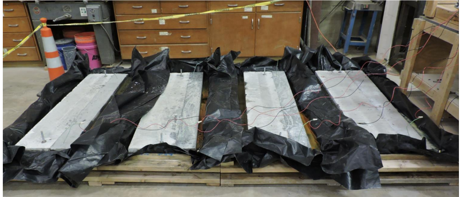
Composite specimens in saline solution during accelerated corrosion testing
