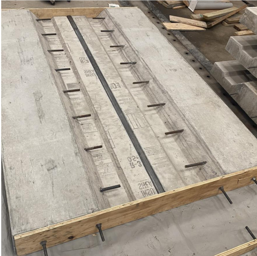
Adjacent panels set up for connection with 2-inch spacer
