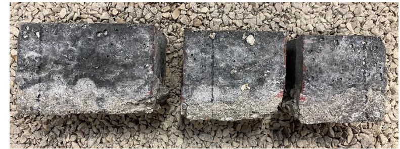
0% fibers specimen after 350 cycles
