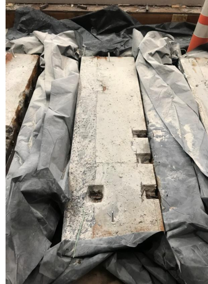
J3 non-proprietary UHPC composite specimen post-corrosion testing with pockets cut out to observe rebar
