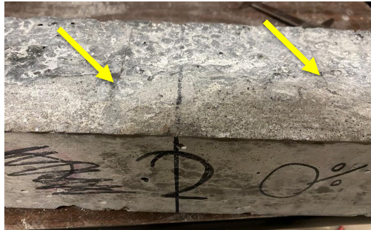
0% fibers specimen after 150 cycles showing transverse cracks
