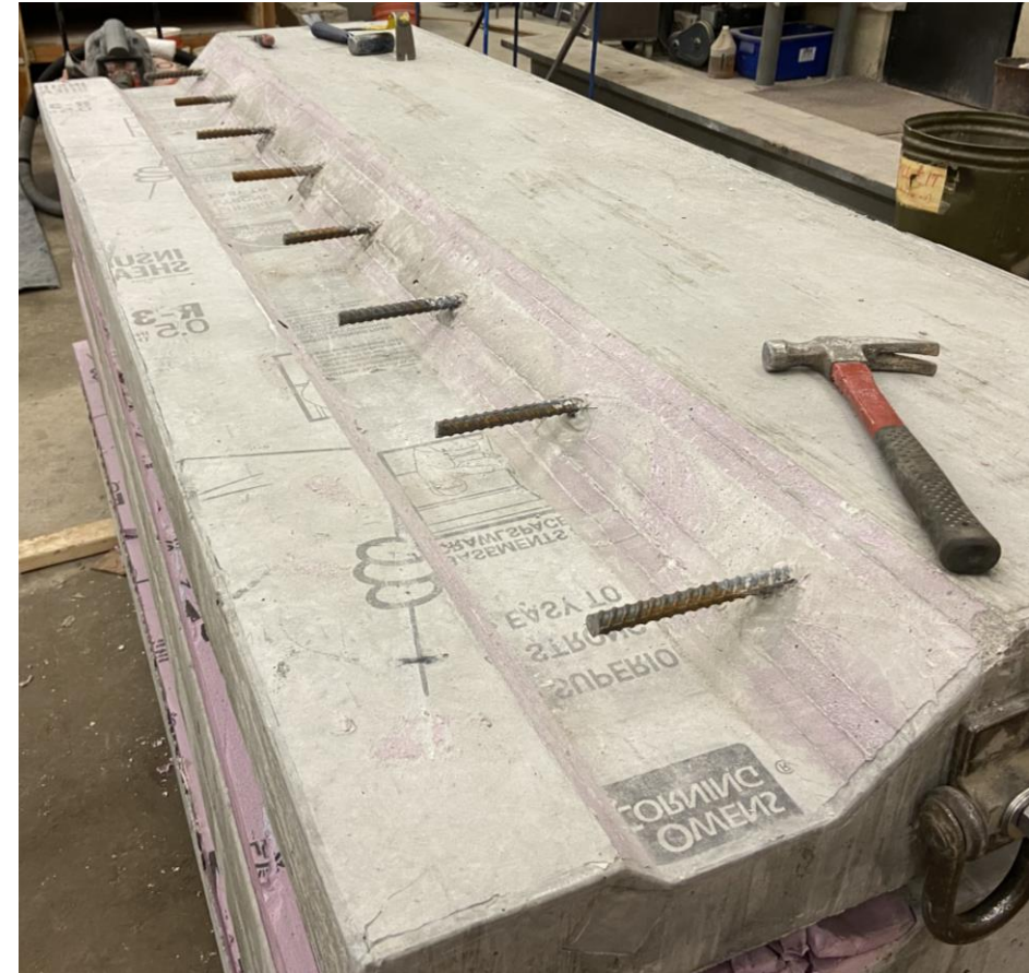
Concrete panel with foam insert removed, exposed rebar
