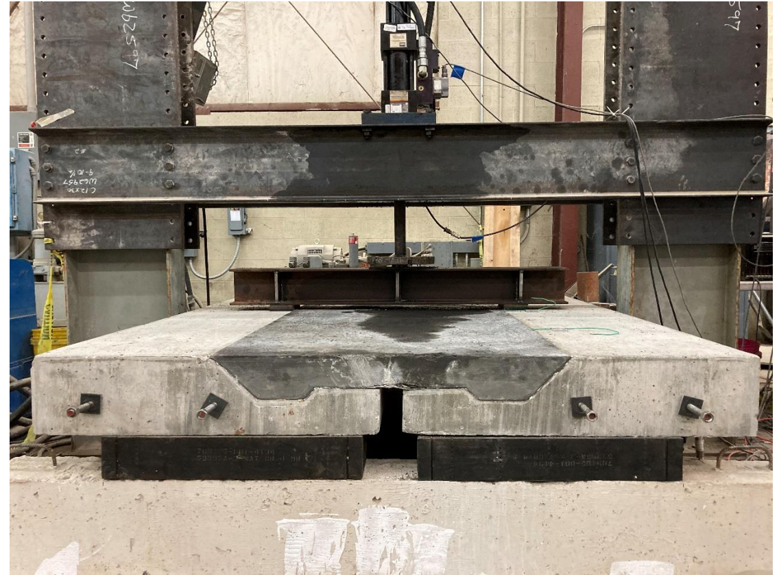
J3 non-proprietary UHPC link slab in compression loading
