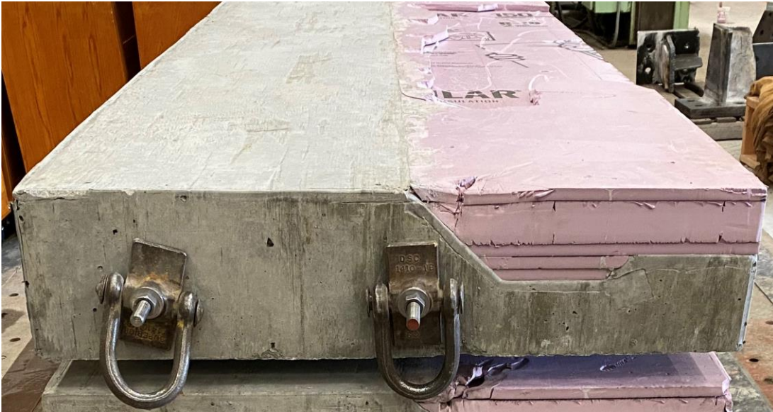
Concrete panel removed from formwork and flipped
