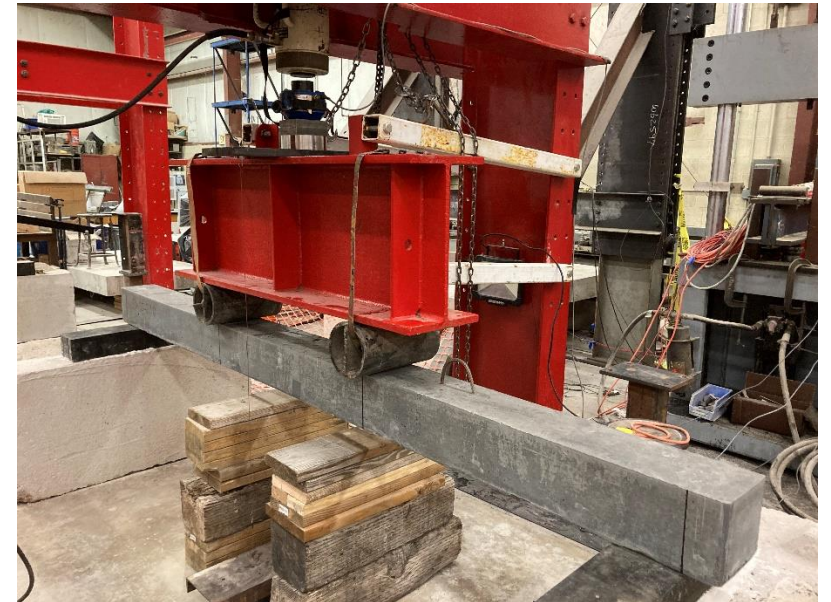
Splice beam testing arrangement
