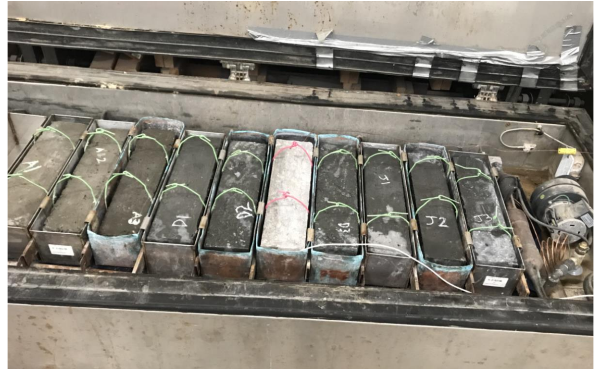
UHPC specimen sections in freeze-thaw machine
