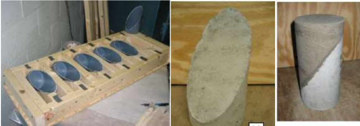
Figure 40: Bond strength test between grout and concrete (Scholz et al., 2007)
