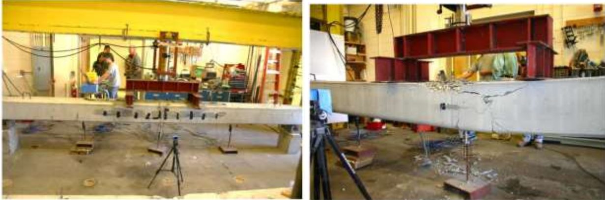
Figure 31: Bending testing of scaled spliced pile specimen (Mullins & Sen, 2015)
