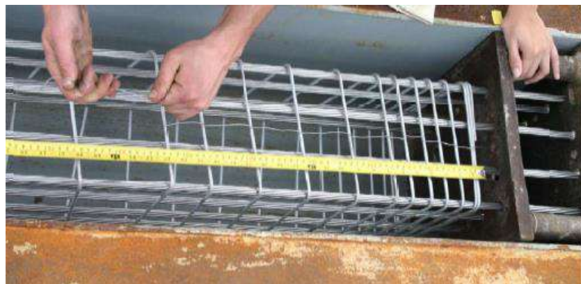
Figure 11: PPCP with Stainless Steel Strand and Spiral (Mullins et al., 2014)
