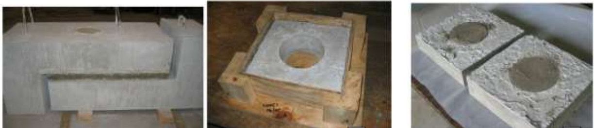
Figure 39: The tests for grouts that fill the haunch between the top of a beam and the bottom of a deck panel
