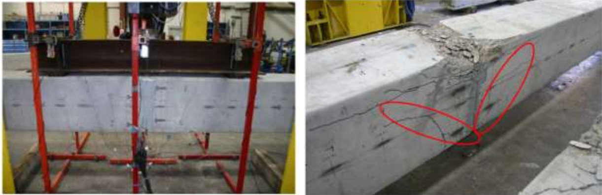
Figure 32: Bending testing of full-scale spliced pile specimen (Mullins & Sen, 2015)
