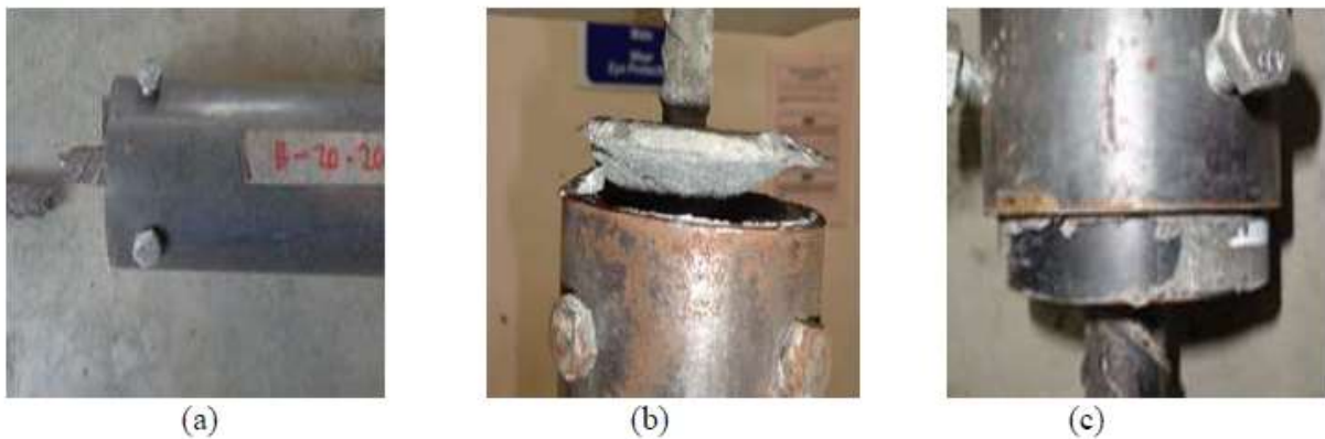
Figure 56: Modes of failure: (a) bar fracture (b) bar pull out (c) internal sleeve-grout failure (Alias et al., 2014)
