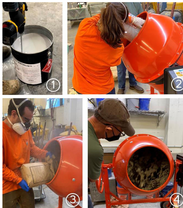
Fig. 1. Laboratory mixing process for HCSC (1) addition of initiator and accelerator to binder resin, (2) addition of binder to mixer, (3) addition of aggregates and fibers to mixer, (4) mixing
