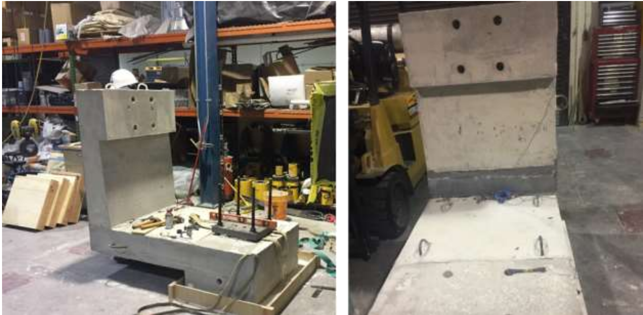
Figure 8- Constructed specimens, cast-in-place barrier (left) and prefabricated barrier with UHPC connection (right).
