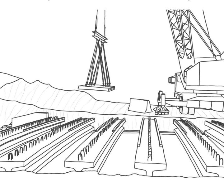
Using prefabricated elements and systems in ABC, such as precast concrete deck panel elements being installed here, can make bridges easier to construct, especially when they are over railroads, rivers, and other roadways.
