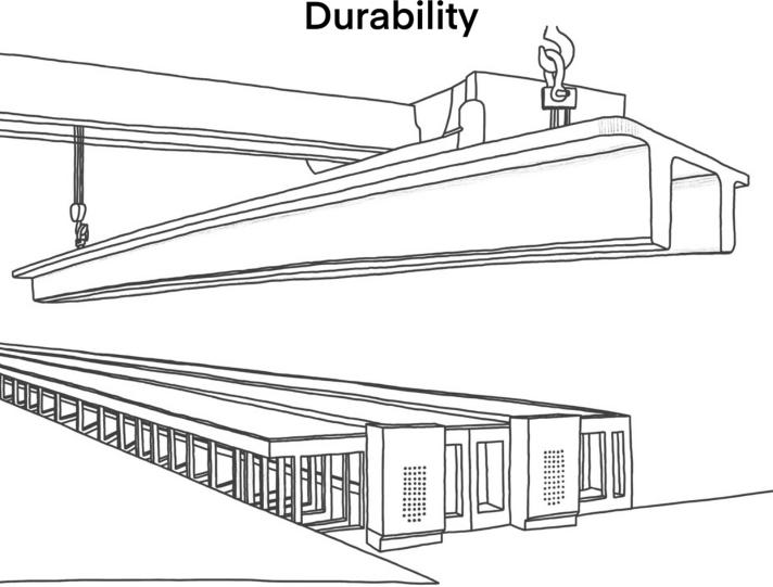
Constructing a bridge on site to a high degree of quality can be challenging, given the harsh environments in which work crews can be exposed. Better material and quality control in prefabrication facilities, as shown here, leads to improved quality and long-term durability for prefabricated elements.
