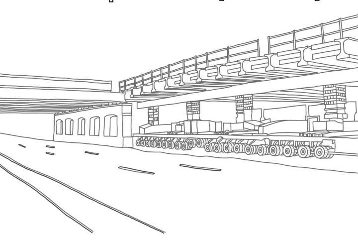
SPMTs are very large computerized platforms that can be used to move entire bridges. A bridge can be replaced in just a few hours with the help of SPMTs. SPMTs can move full bridges that weigh over 33 million pounds!
