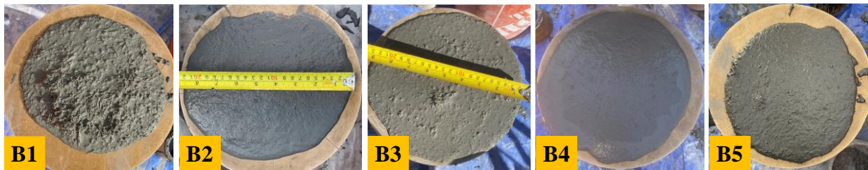
Figure 2-4: Static flow of the fresh NP-UHPC mixes.
