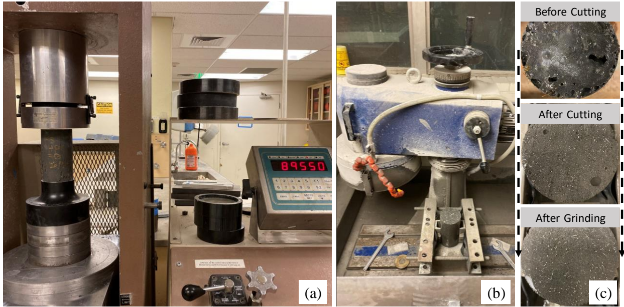
Figure 2-5: Compression testing of NP-UHPC cylinders: (a) test setup; (b) grinding machine for cylinder preparation; and (c) views of typical NP-UHPC cylinder through preparation sequence.
