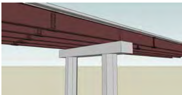
▼ Continuous girder with bolted splices.
