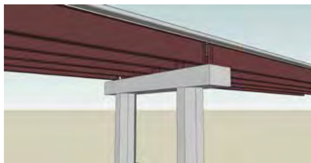
▼ Simple-span bridge with joint-less deck.
