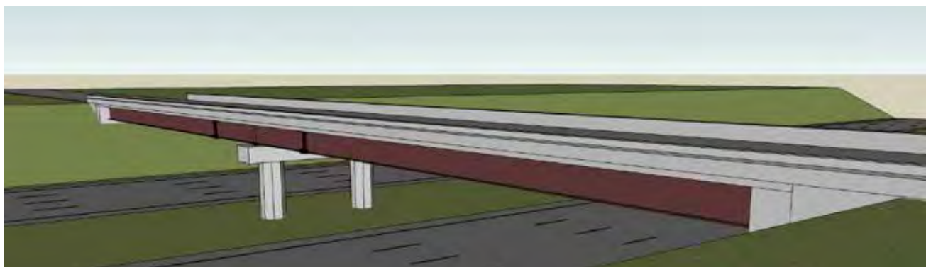
▲ Typical two-span overpass bridge.
